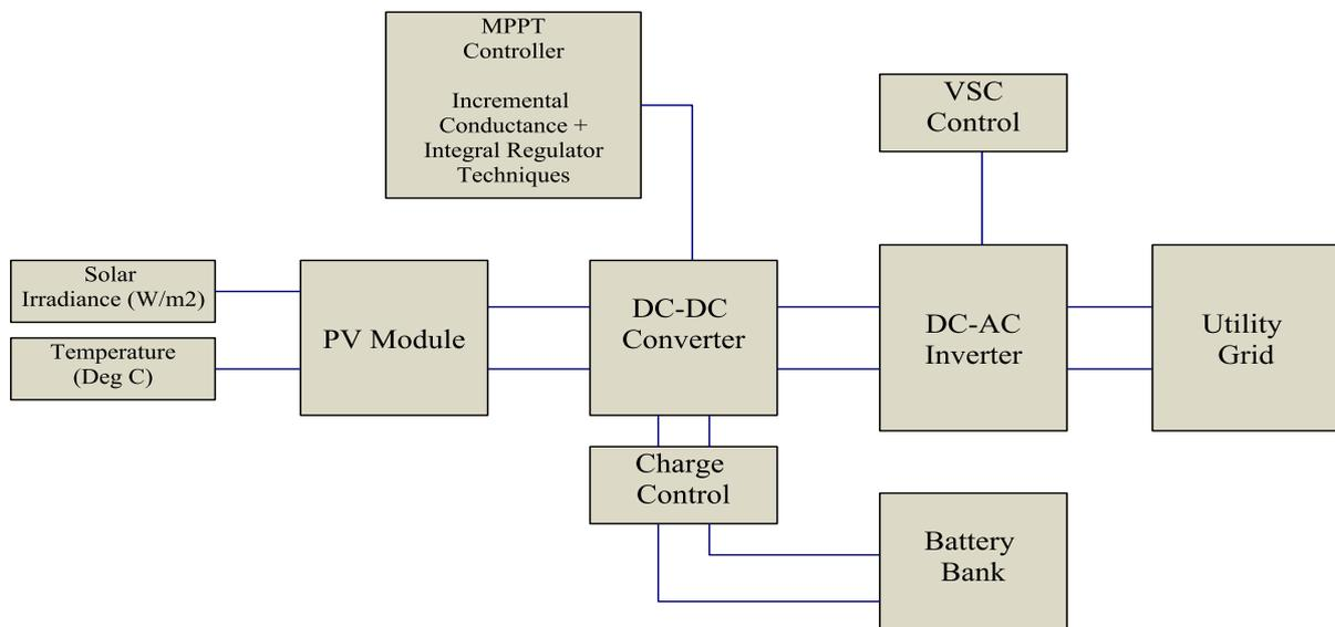
**Figure 1. Photovoltaic system model producing power (kWh) proportional to global solar irradiance and temperature (°C) data**
