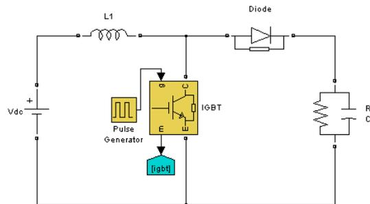
**Figure 5. DC-DC boost converter with MPPT control**
