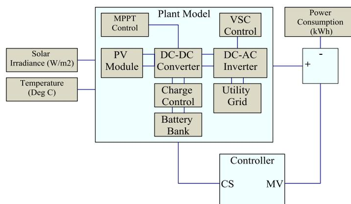
**Figure 8. Plant model with controller**
