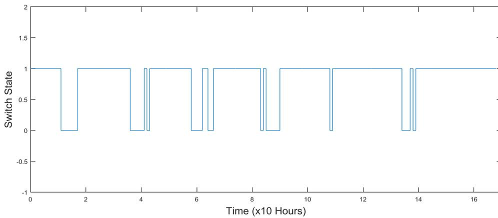
**Figure 12. Control switch states for demand more than PV production**
