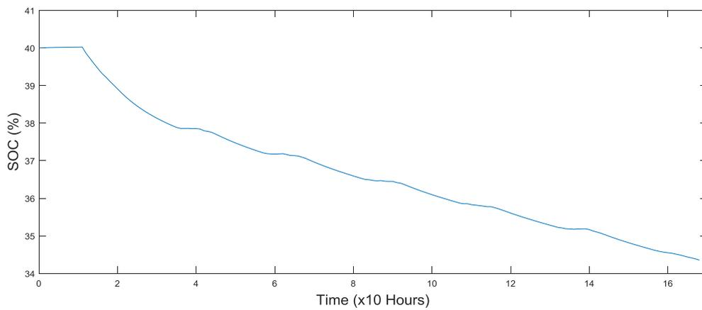
**Figure 13. Lead acid battery SOC showing charging and discharging behaviour**
