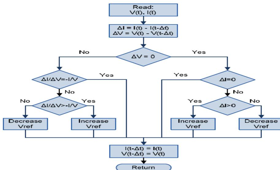
**Figure 4. Flowchart of the IC Algorithm**
