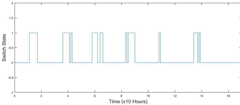
**Figure 11. Control switch states for PV production more than demand**
