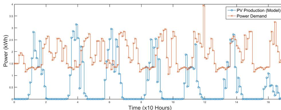
**Figure 10. Modelled output power and real load for 3KW system installed in New Plymouth**
