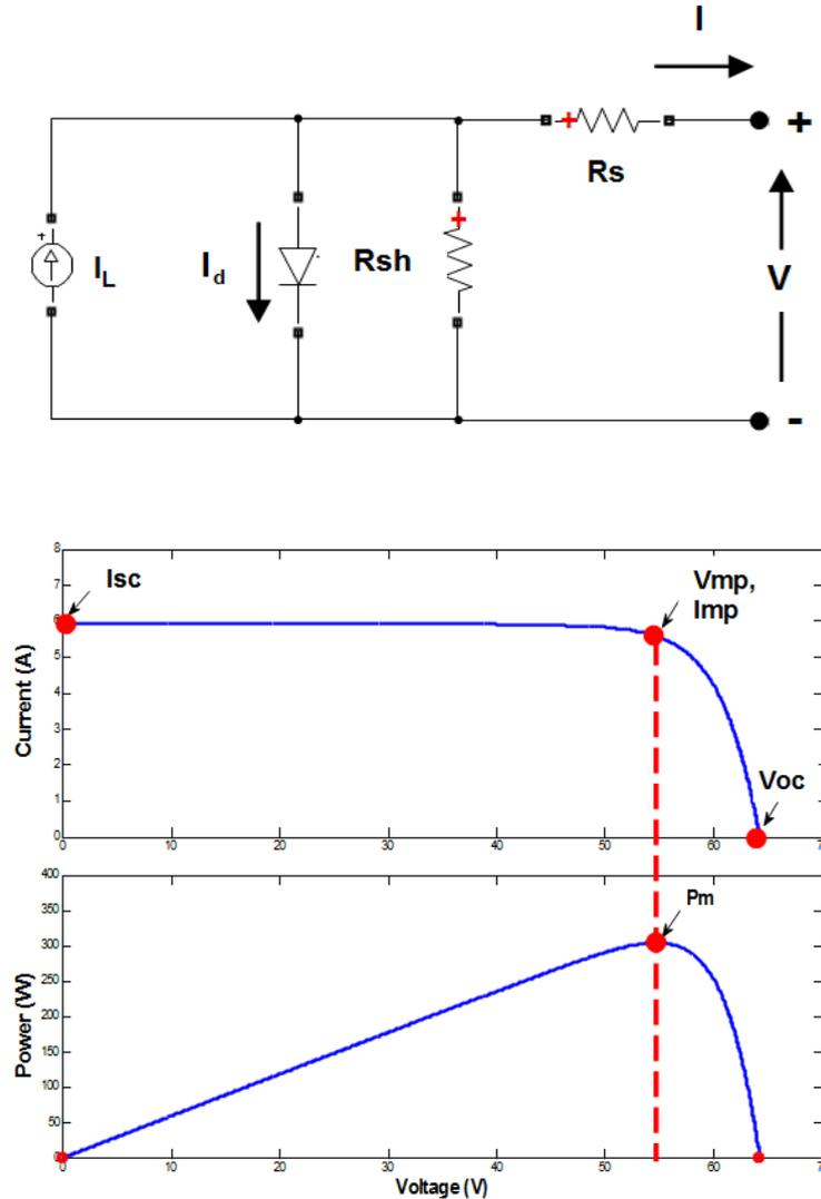
Figure 2. Single diode model of a solar cell, current and power characteristic curves
