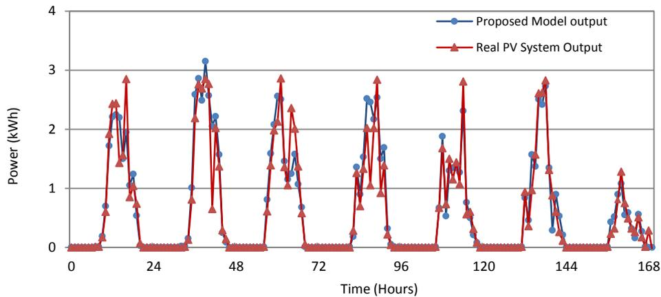
**Figure 9. Output power of proposed model vs real 3KW system installed in New Plymouth**
