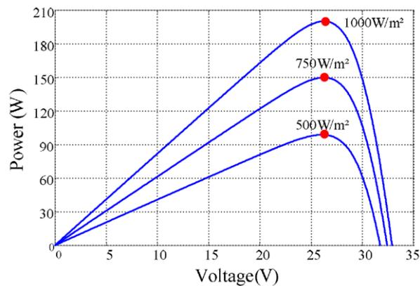
**Figure 3. Power characteristic for different levels of irradiation**
