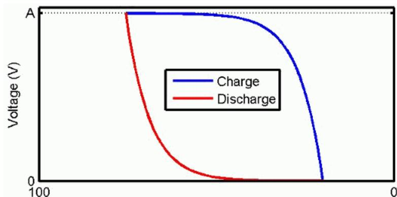
**Figure 7. Exponential zone for Lead\_Acid battery, State of charge (%)**
