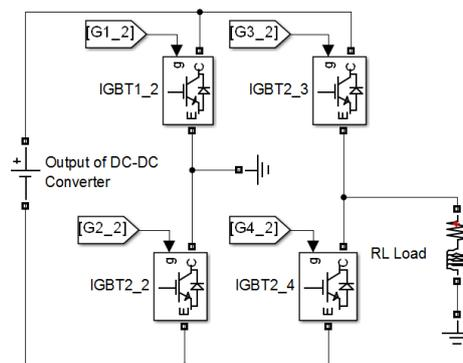
**Figure 6. Single phase full-bridge inverter**
