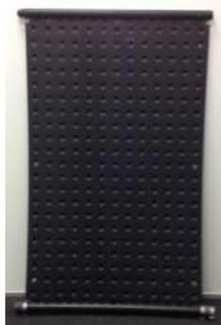
**Figure 1. (a) Prototype collector, (b) pillow absorber in prototype collector**
