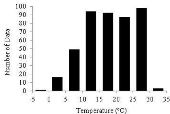
**Figure 5. Frequency histogram of the difference between the average module temperature and the ambient temperature when POA irradiance  $> 200 \text{ W/m}^2$**
