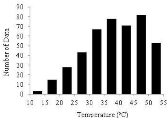
**Figure 4. Frequency histogram of the average temperatures of all 5 modules for POA irradiance  $> 200 \text{ W/m}^2$**
