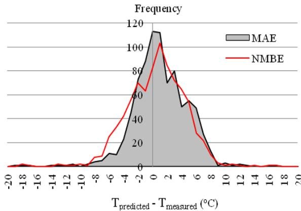
**Figure 9. Frequency distributions of errors in prediction of SNL's model by MAE and NMBE methods relative to measured temperatures**
