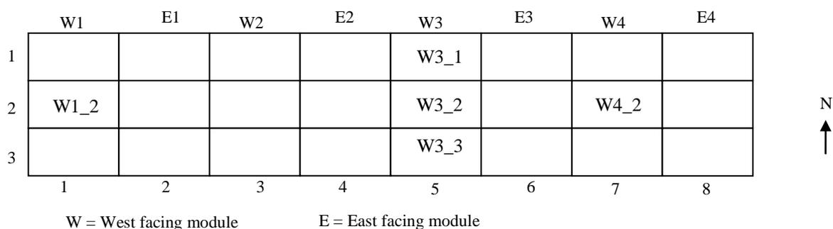
**Figure 3. The layout of temperature sensor positions**
