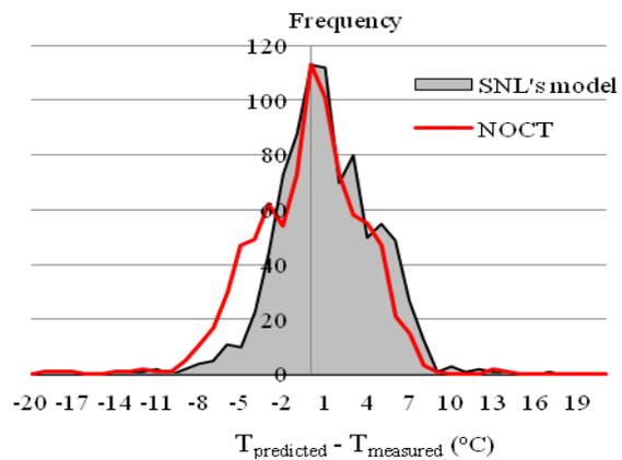
**Figure 10. Frequency distributions of the difference between predicted and measured modules temperature of SNL's temperature model and NOCT**
