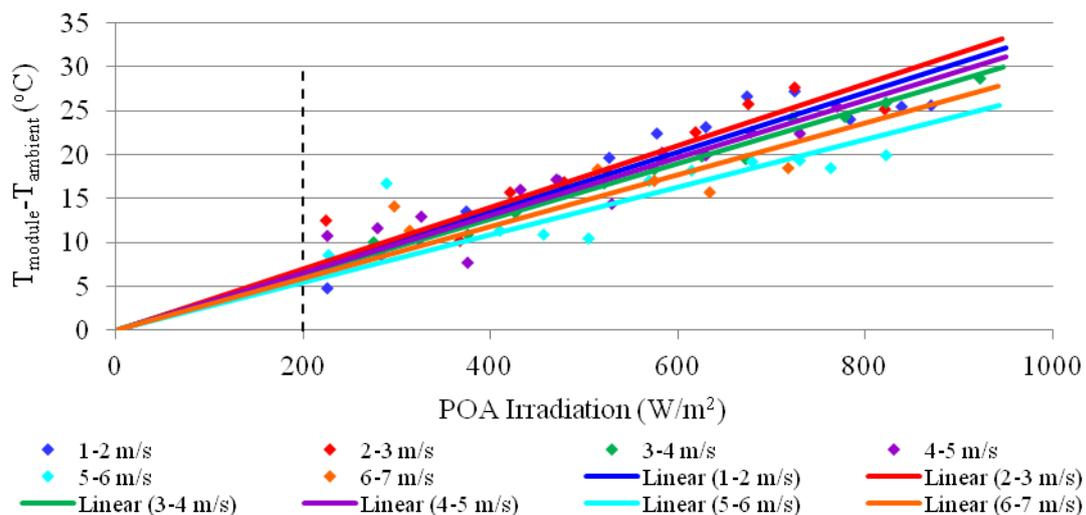
**Figure 6. Difference between the average module temperatures and the ambient temperature as a function of POA irradiance categorised by wind speed bin. The data is the average of the difference in temperature within an irradiance bin of 50 W/m<sup>2</sup>.**
