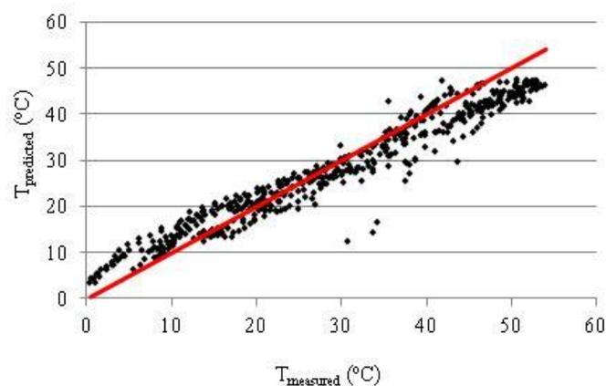
**Figure 8. Plot of predicted temperature by NOCT and measured temperature**
