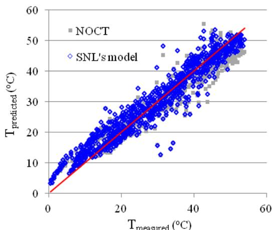
**Figure 11. Plot of predicted against measured module temperatures between NOCT and SNL's temperature model.**
