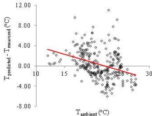
**Figure 12. Scatter plot of the difference between predicted and measured module temperature of SNL's temperature model as a function of ambient temperature. (A red line is added to show the trend.)**
