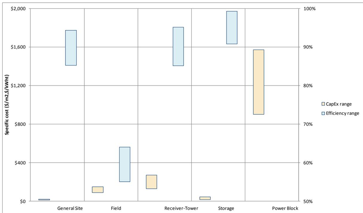
**Figure 3. Cost and performance ranges for components of the system with a 50% efficient power block**
