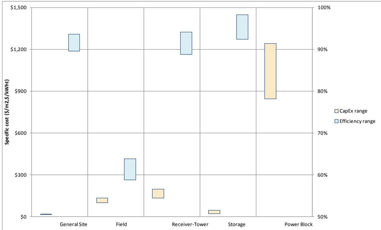
**Figure 1. Cost and performance ranges for components of the system with a 42% efficient power block**
