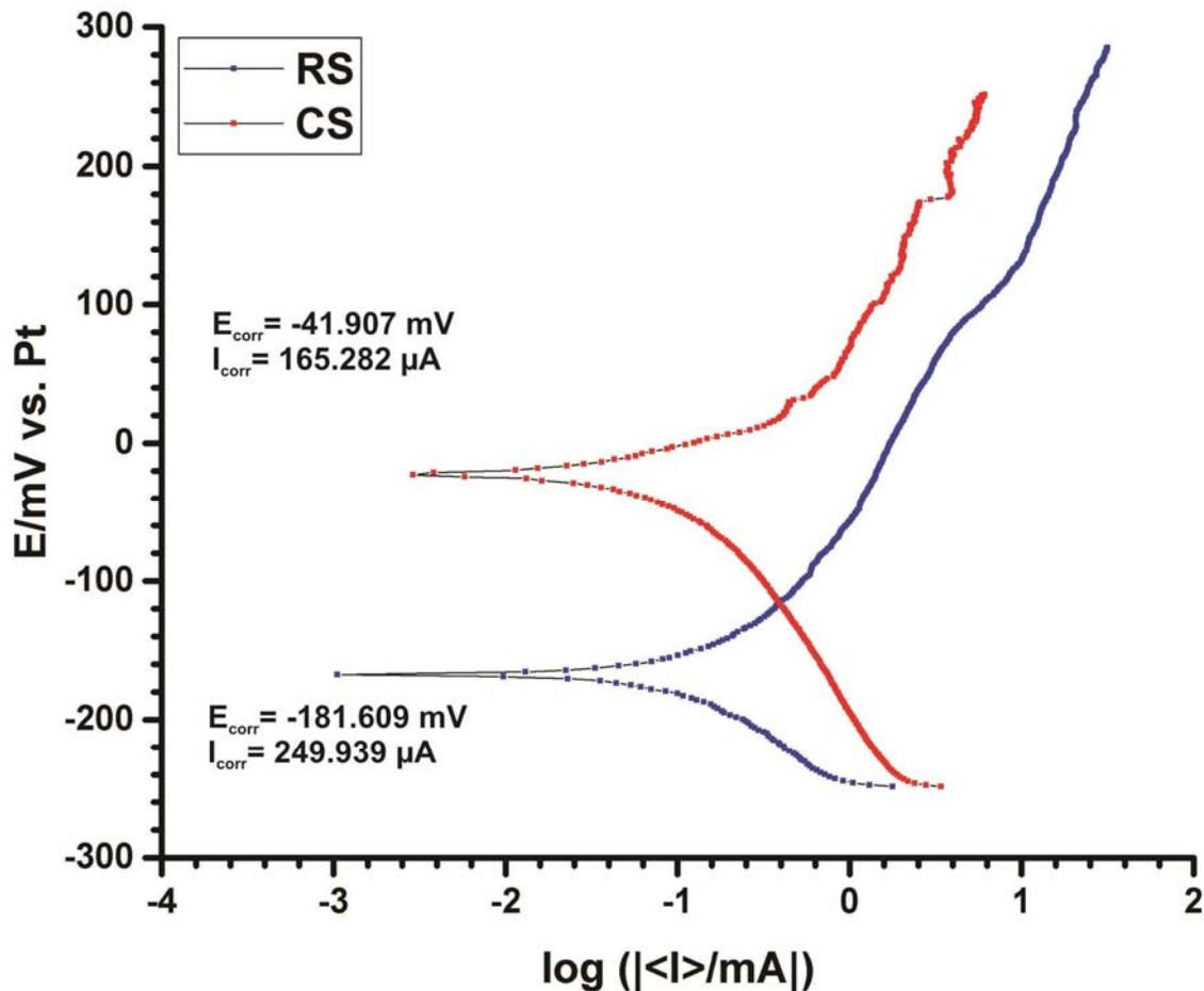
**Figure 7. Potentiodynamic polarization curves comparing corrosion behaviour between RS and CS in the eutectic salt at 450°C**
