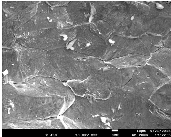
**Figure 2. SEM-SE micrograph of the fracture surface showing 100% grain boundary crack morphology and salt residue**
