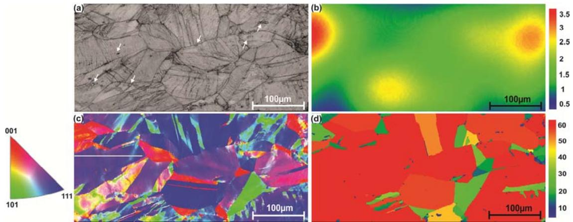
**Figure 4. (a) Band contrast, (b) strain contouring map, (c) IPF X colour map, (d) maximum orientation spread map (MOS) of the same area in RS. White arrows in (a) point to dispersed Ti-rich particles in the matrix; accelerating voltage= 30 kV, step size= 0.5  $\mu\text{m}$**
