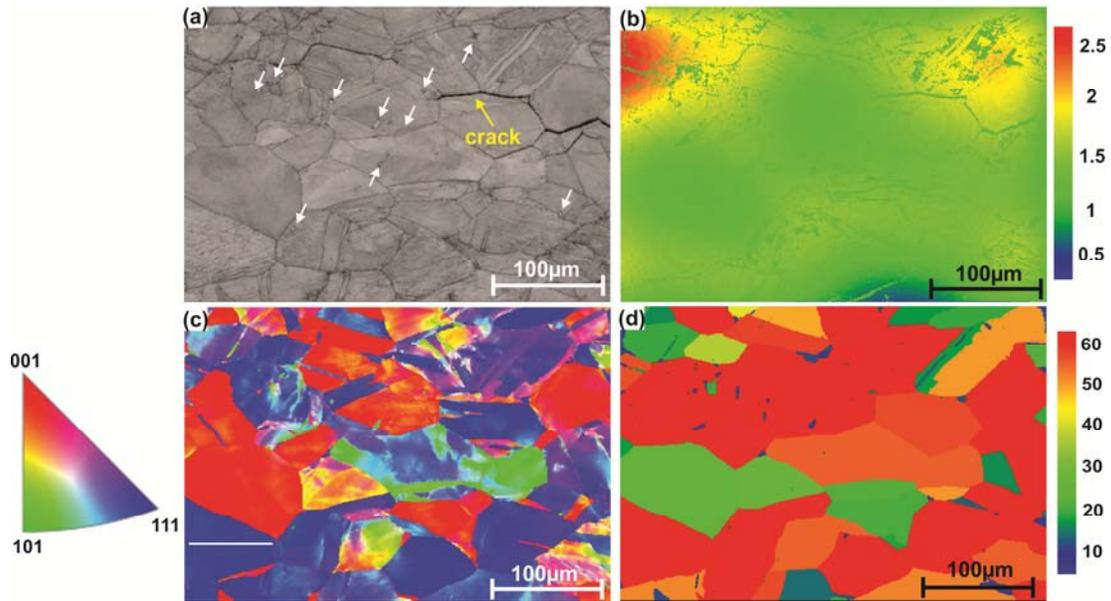
**Figure 3. (a) Band contrast, (b) strain contouring map, (c) IPF X colour map, (d) maximum orientation spread map (MOS) of the same area in the cracked specimen (CS) including crack tip (yellow arrow). White arrows in (a) point to dispersed Ti-rich particles in the matrix; accelerating voltage= 25 kV, step size= 0.65  $\mu\text{m}$**
