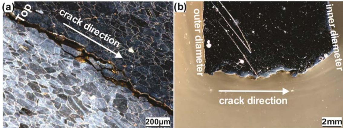
**Figure 1. (a) Micro-graph image of the cracked crucible showing crack initiation area, top part of the crucible and growing direction downwards (etched sample), (b) top view macro-graph of the crucible sidewall showing outer and inner diameters and crack growth direction across the crucible wall (un-etched sample)**
