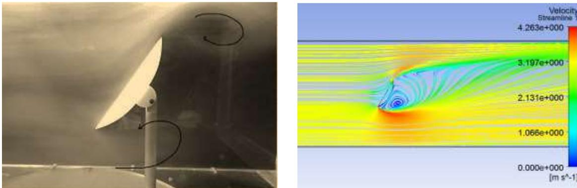
Fig 3: Flow visualization and stream lines for  $60^\circ$  tilt angle
