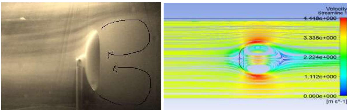
Fig 10: Flow visualization and stream lines for  $-90^\circ$  tilt angle
