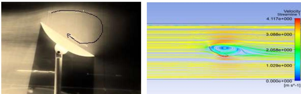
Fig 7: Flow visualization and stream lines for  $-30^\circ$  tilt angle
