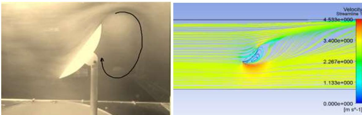
Fig 4: Flow visualization and stream lines for  $45^\circ$  tilt angle
