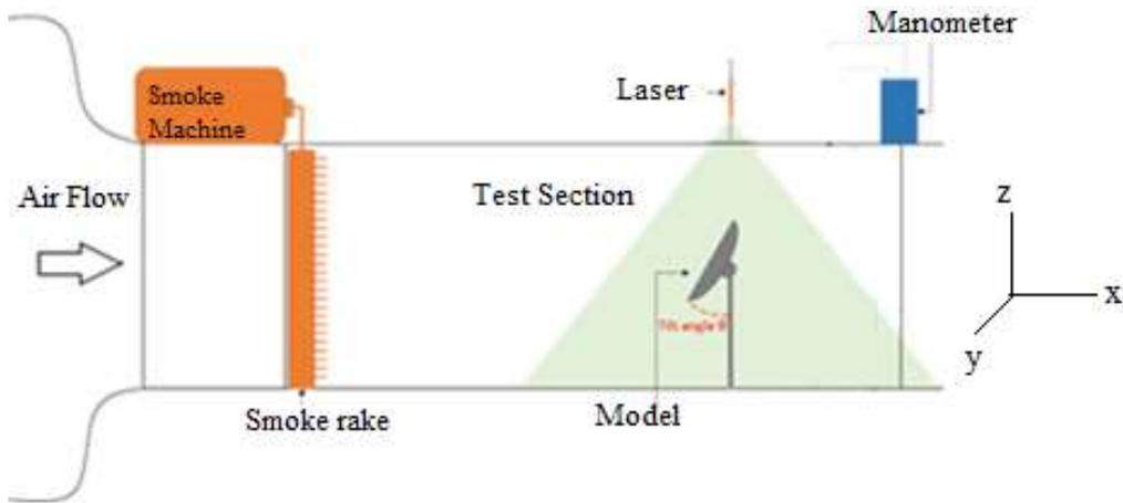
Fig 1: Schematic drawing of the experimental bench
