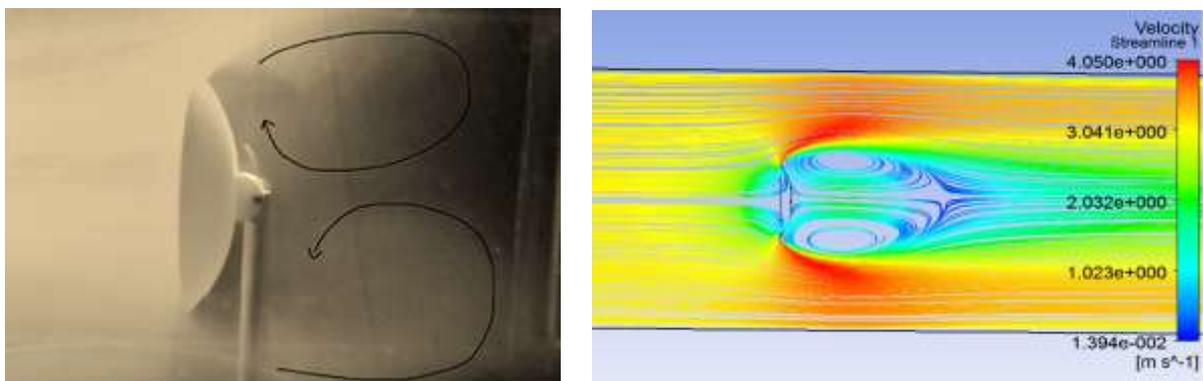
Fig 2: Flow visualization and stream lines for  $90^\circ$  tilt angle
