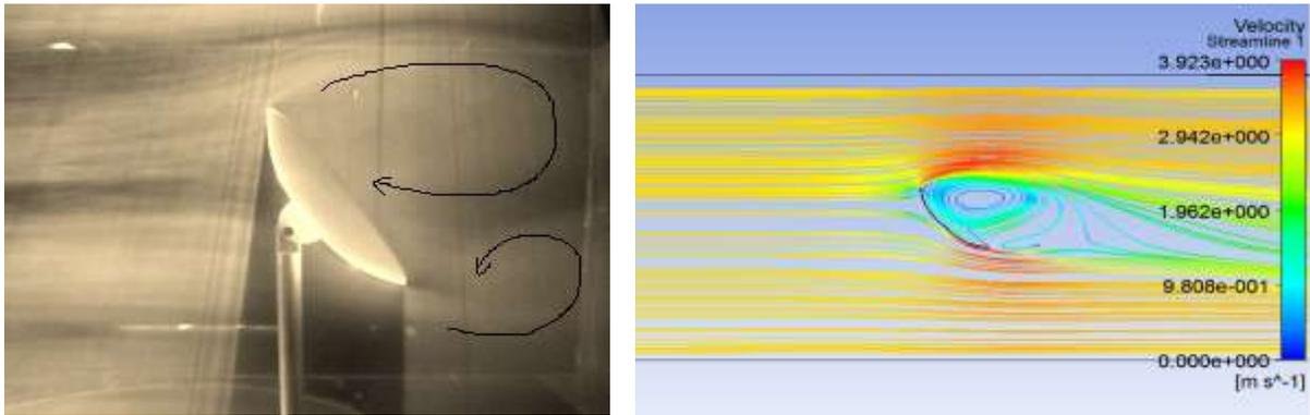
Fig 8: Flow visualization and stream lines for  $-45^\circ$  tilt angle
