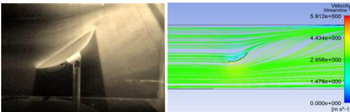
Fig 5: Flow visualization and stream lines for  $30^\circ$  tilt angle
