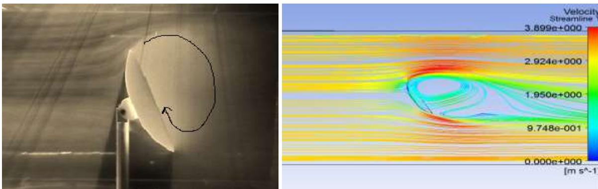
Fig 9: Flow visualization and stream lines for  $-60^\circ$  tilt angle
