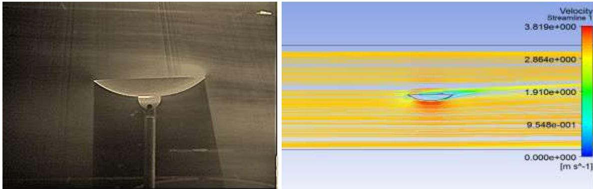
Fig 6: Flow visualization and stream lines for 0° tilt angle
