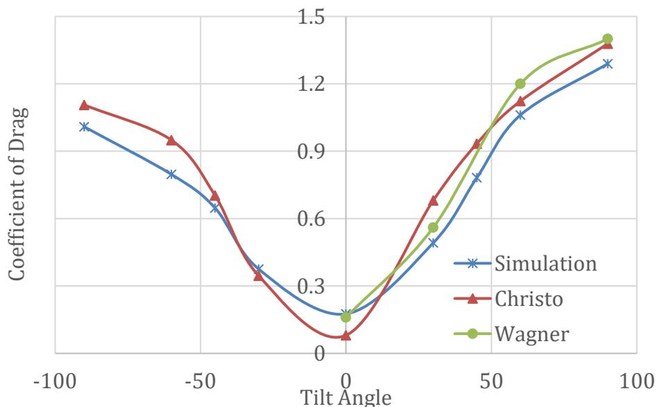
Fig 11: Comparison of drag coefficient at different tilt angles
