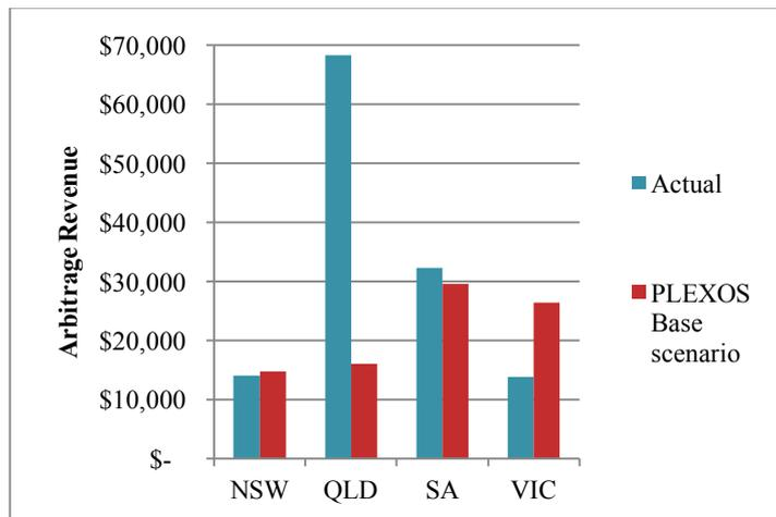
**Figure 3. FY2014-15 arbitrage revenue for 1 MW / 1 MWh battery – comparison of actual pricing data and PLEXOS results**
