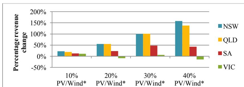
**Figure 10. Percentage revenue change from Base scenario for PV/wind capacity penetration scenarios (\*existing SA wind penetration kept at 29%, VIC penetration kept at 7% for 10% PV/wind scenario)**
