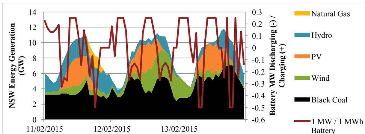
**Figure 8. Typical 3-day summer period showing hourly generation in NSW, and the charge/discharge profile of a 1 MW / 1 MWh battery performing arbitrage – 40% PV/wind capacity penetration scenario**
