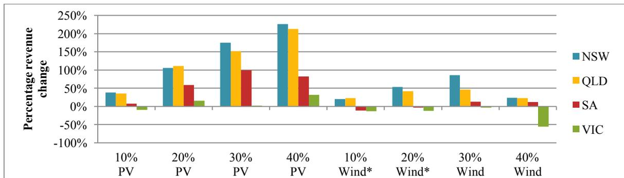
**Figure 9. Percentage revenue change from Base scenario for PV and wind capacity penetration scenarios (\*existing SA wind penetration kept at 29%)**
