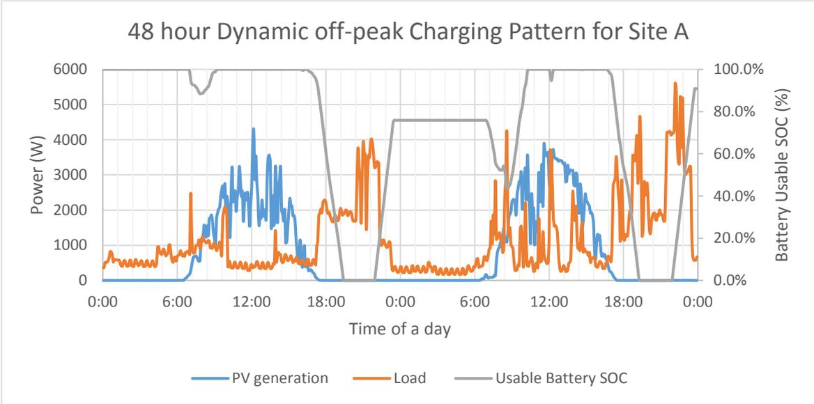
**Figure 6: 48 hour Dynamic off-peak charging pattern for Site A, utilising a 6 kWh battery system**
