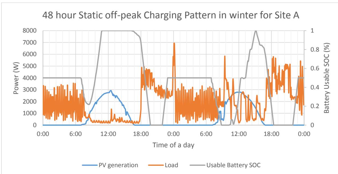
**Figure 5: 48 hour 50% Static off-peak charging pattern for Site A, utilising a 6 kWh battery system**
