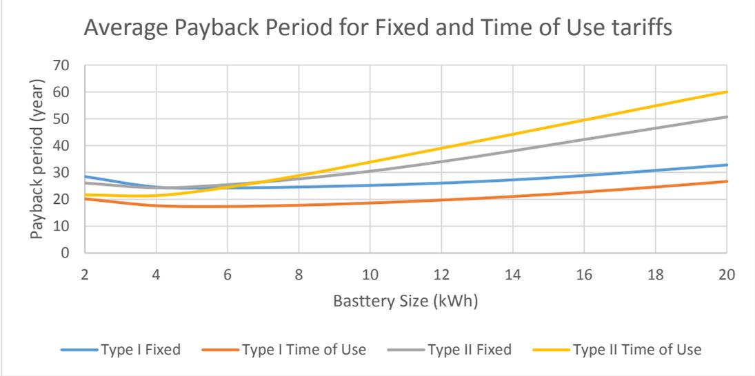
**Figure 7: Average payback period of different battery sizes for Type I and Type II sites with both Fixed and Time of Use tariffs**
