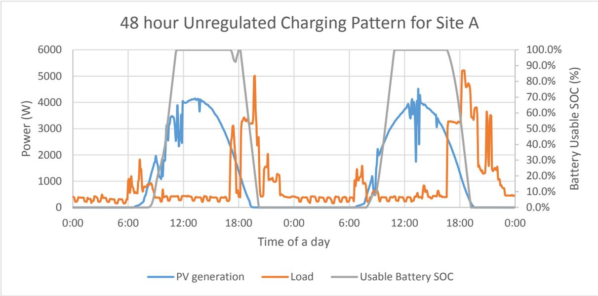
**Figure 3: 48 hour Unregulated Charging Pattern for Site A, utilising a 6 kWh battery system**
