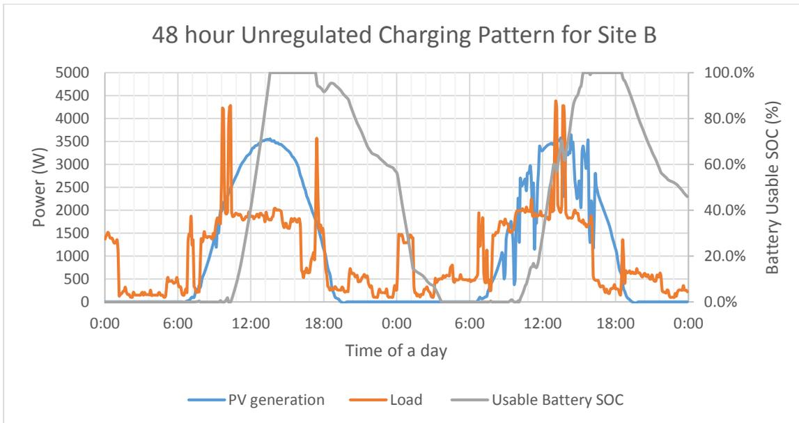
**Figure 4: 48 hour Unregulated charging pattern for Site B, utilising a 6 kWh battery system**
