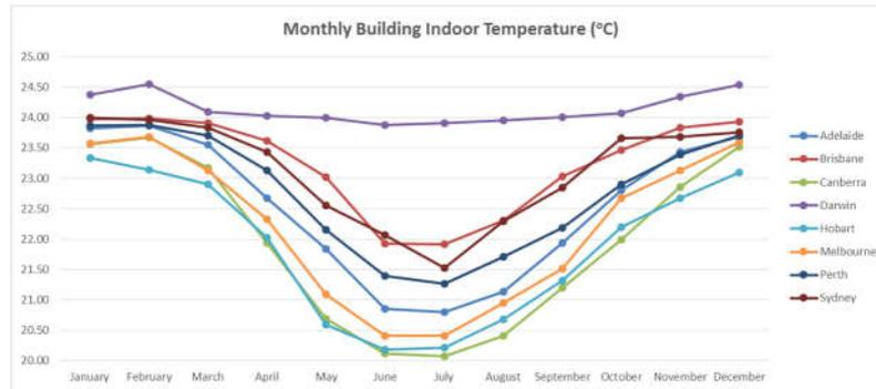
**Figure 3. Monthly building indoor temperature for SDEC-ST system**
