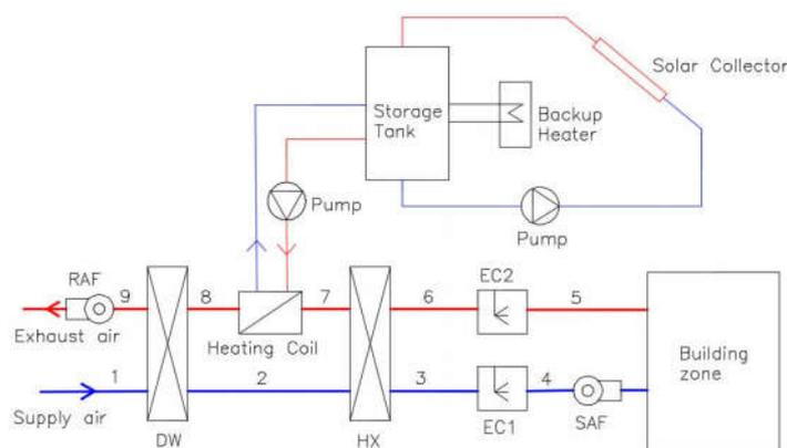
**Figure 2. Schematic diagram of the SDEC system**
