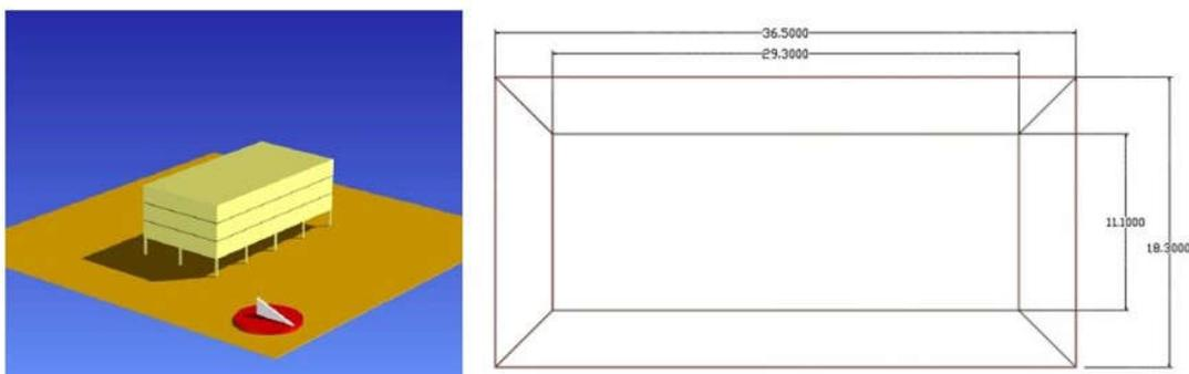
**Figure 1. Building model geometry and zone division**
