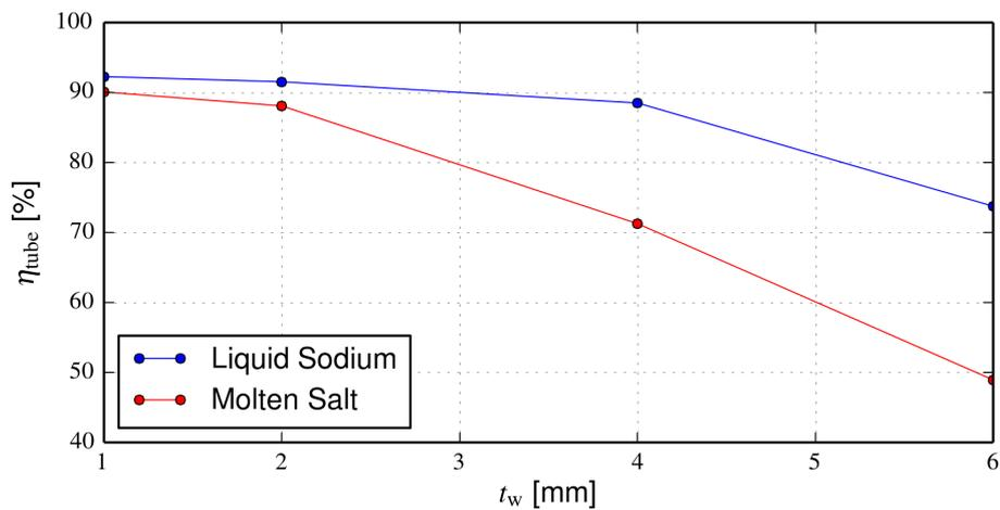
**Figure 7:** Plot of **Inconel® 625LCF** tube efficiency for both liquid sodium and molten salt with increasing tube thickness
