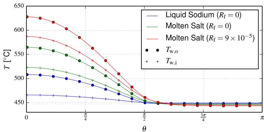
**Figure 4:** Circumferential temperature of an [Inconel® 625LCF](#) tube irradiated with  $CG = 800 \text{ kW/m}^2$
