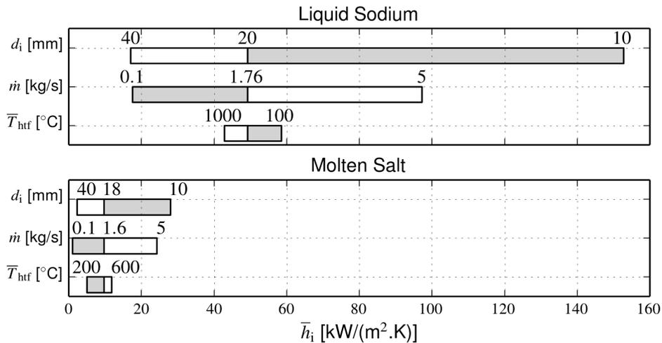
**Figure 2:** Tornado chart showing the dependency of convective heat transfer coefficient  $\overline{h}_i$  on tube diameter  $d_i$ , mass flow  $\dot{m}$  and bulk fluid temperature  $\overline{T}_{\text{htf}}$  for both liquid sodium and molten salt
