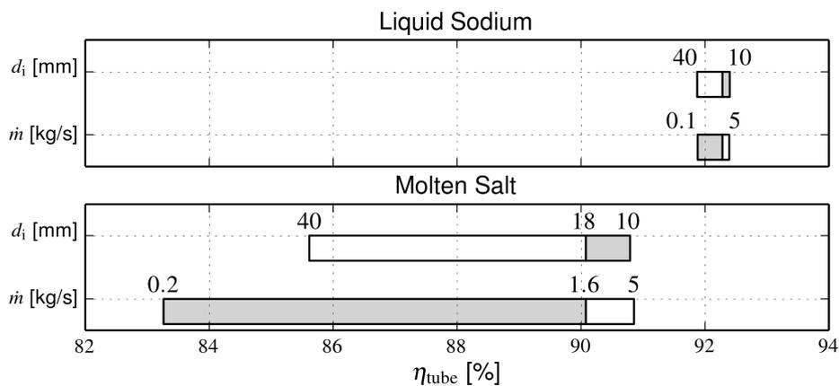
**Figure 5:** Tornado chart showing the dependency of Inconel® 625LCF tube efficiency on tube diameter  $d_i$  and mass flow  $\dot{m}$  for both liquid sodium and molten salt
