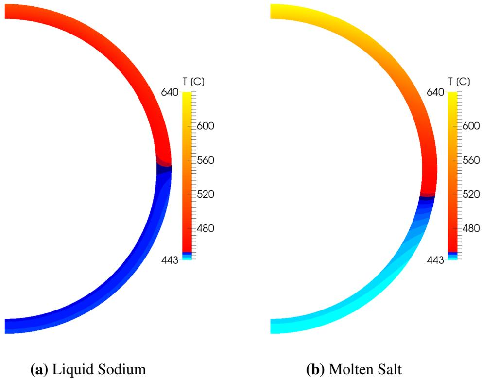
**Figure 6:** Screenshots from **ParaView** showing tube temperature with molten salt and liquid sodium as in Table 1
