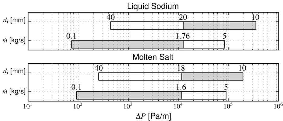
**Figure 3:** Tornado chart showing the dependency of pressure drop on tube diameter  $d_i$  and mass flow  $\dot{m}$  for both liquid sodium and molten salt
