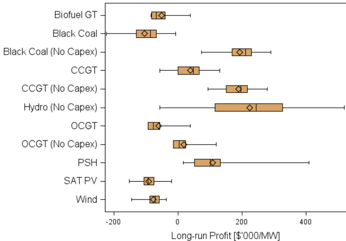
**Figure 2. Box plots of generator long run profitability by technology type annually, single outage trace. Whiskers show full range of observations.**
