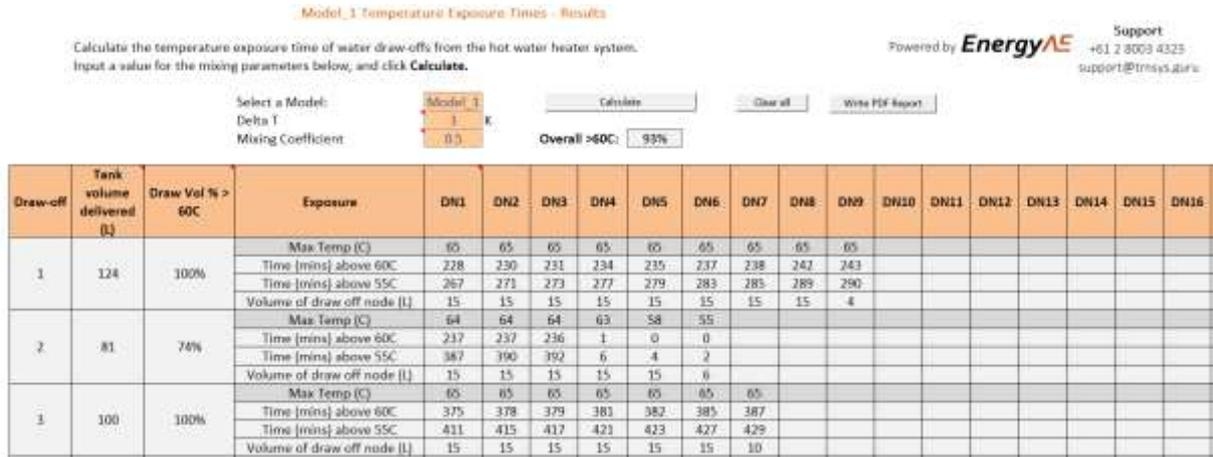
Table 1 shows the simulation results for ‘Model\_1’. The animation next to the simulation results plot below in Figure 4 is shown at the start of the simulation, time = 0 hours. The temperature at each node is equal to the initial tank temperature specified in the model setup in Figure 1. In the excel interface, the user may step through the results in time and view the animated changing water temperatures in the tank.
