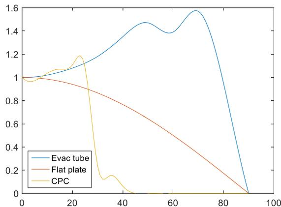
**Figure 3: Indicative IAMs for different collector technologies**
