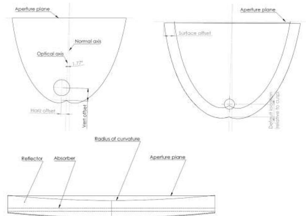
**Figure 4 a-c: Manufacturing deviations as modelled – (a) vertical and horizontal offset of the absorber; (b) offset from the absorber surface; and (c) vertical curvature of the reflector**
