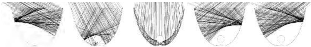
**Figure 2 (a-e): Optical response of a CPC to varying source directions**
