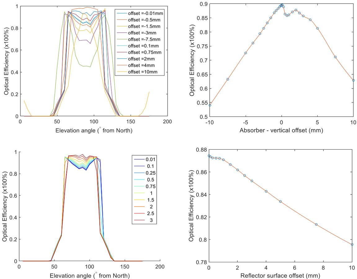
**Figure 6 (a-b): Performance impact of offsetting the absorber vertically; (c) detail of the impact of small movement *downwards*; and (d) Performance impact of offsetting the reflector surface**
