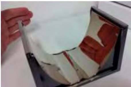
**Figure 8: Aluminium metalised plastic CPC**
