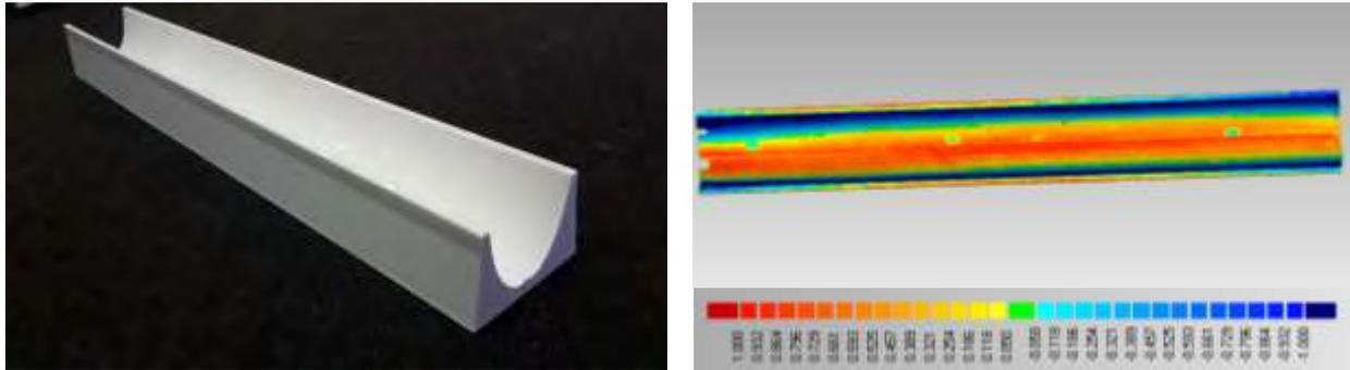
**Figure 9 (a) The mould pattern; and (b) scan results of the fibreglass part**
