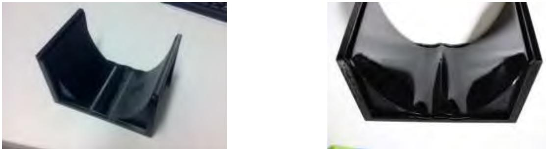
**Figure 7: 3D printed plastic CPC (a) showing the print lines resulting from the printing process; and (b) painted with 2-pack polyurethane (high gloss black) in preparation for vapour deposition of the aluminium reflective surface**
