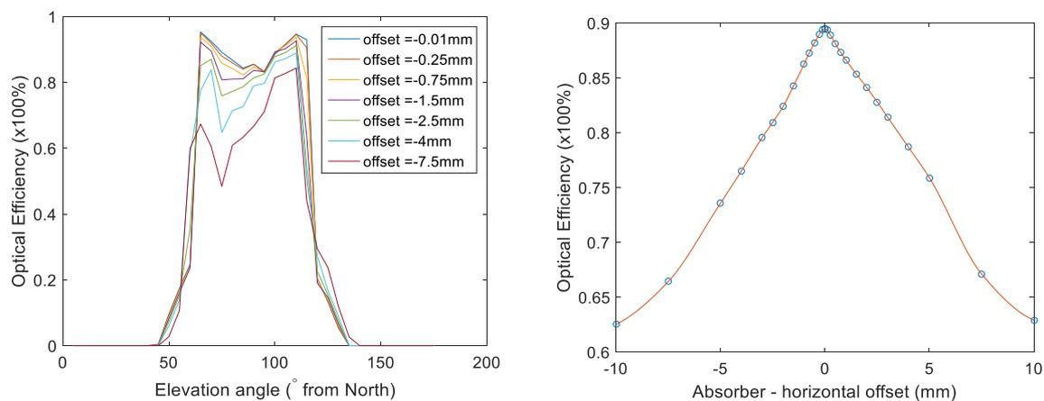
**Figure 5 (a-b): Performance impact of offsetting the absorber horizontally**
