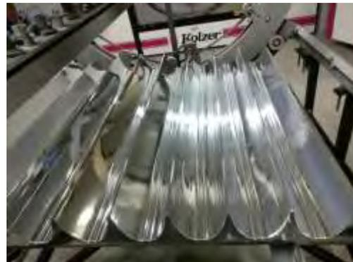
**Figure 11: (a) Scan results of the MDF part; and (b) the final mirrored reflector**
