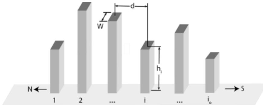
**Figure 1. Nomenclature of a typical 1.5D DSM describing urban features of a relief**
