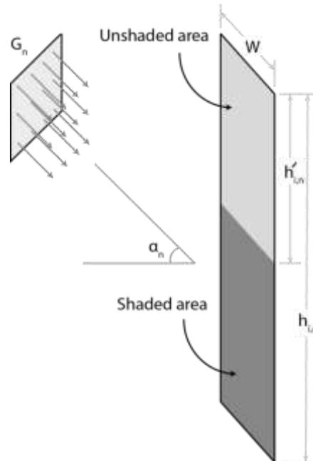
**Figure 3. Solar radiation reaching the surface of a partially shaded feature**
