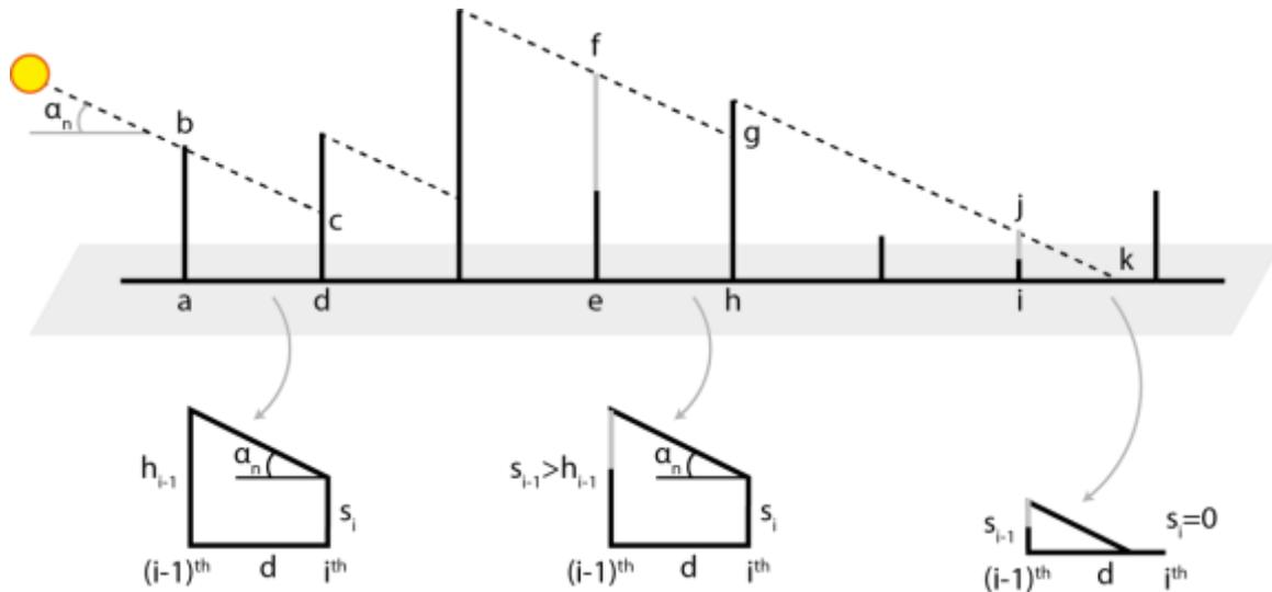
**Figure 2. Shadow cast on features due to sunlight obstructed by the preceding features**
