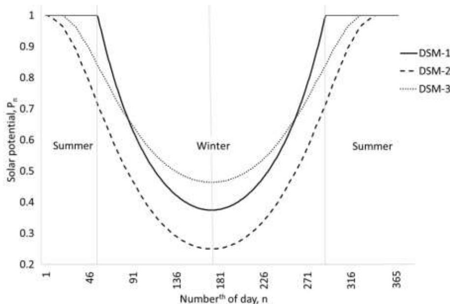
**Figure 5. Comparison of daily solar potential of façades for different layouts**
