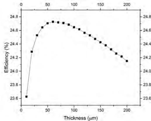
**Figure 4 Variation of simulated efficiency for  $p$ -type IBC solar cell with different cell thicknesses for a fixed bulk minority lifetime and resistivity at 550  $\mu\text{s}$  and 1  $\Omega\text{cm}$ , respectively.**
