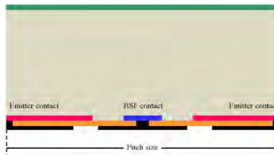
**Figure 6 Cross section of  $p$ -type IBC solar cell with indication of pitch size**
