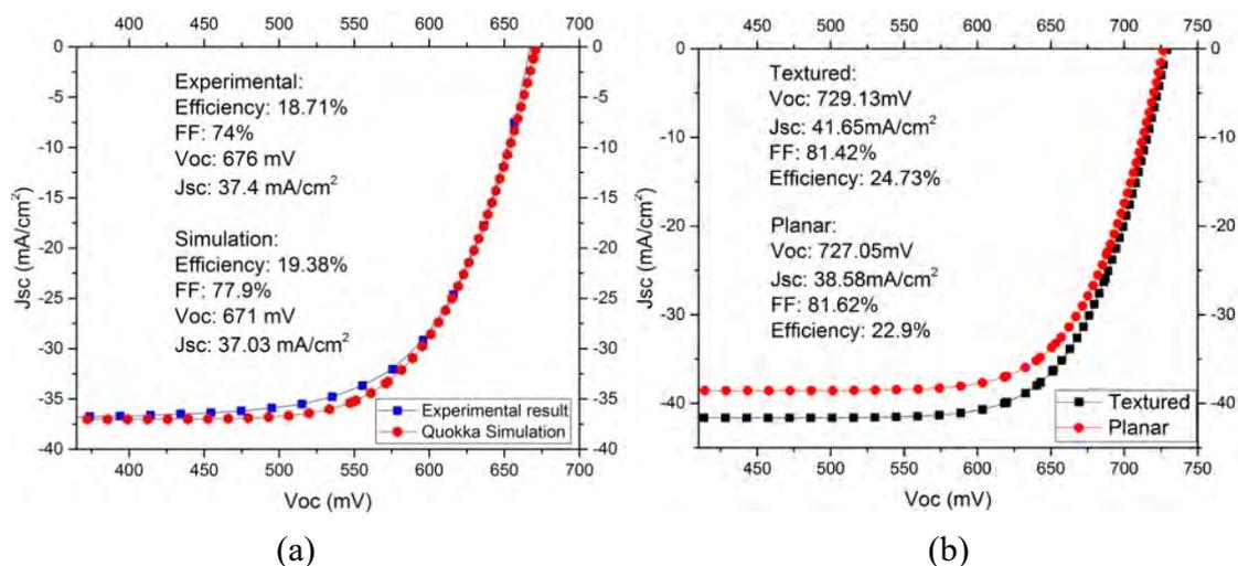
**Figure 2 (a) Simulated and experimental  $J$ - $V$  curves for  $n$ -type IBC solar cell. (b)  $J$ - $V$  curves of a  $60\text{-}\mu\text{m}$   $p$ -type IBC cell with and without front surface texturing.**
