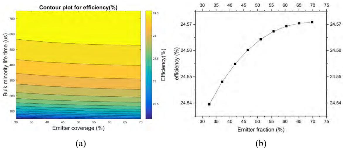
**Figure 8 modelled cell efficiency with (a) combined bulk minority lifetime and emitter fractions (b) only impact on different emitter fractions at fixed lifetime of 550 $\mu\text{s}$**
