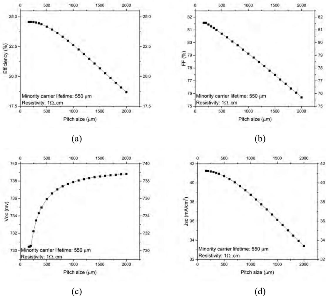
**Figure 7 Quokka simulation results for cell efficiency, Fill-factor, open circuit voltage and short circuit current for different pitch size.**
