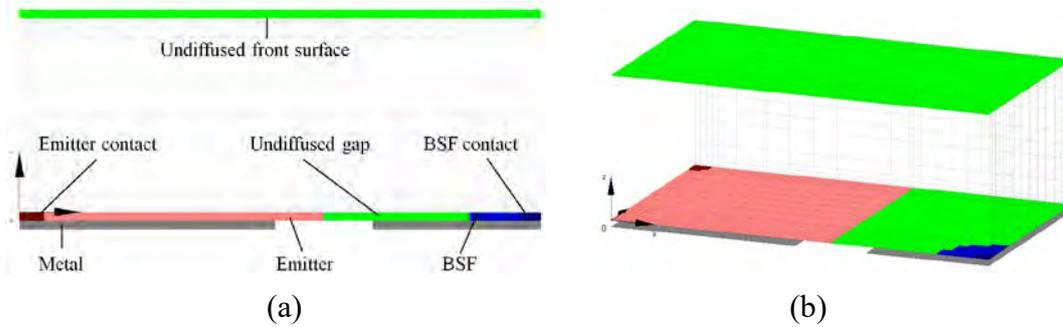
**Figure 1 Schematic of  $p$ -type IBC silicon unit-cell with planar front surface (a) in two-dimensions and (b) in three-dimensions**
