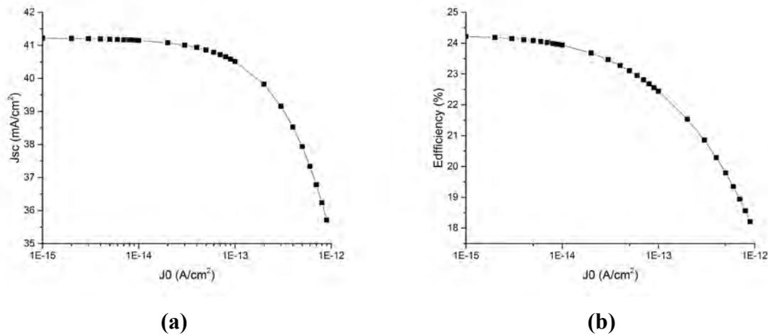
**Figure 5(a) simulated short circuit current density and (b) efficiency as a function of front surface  $J_0$**
