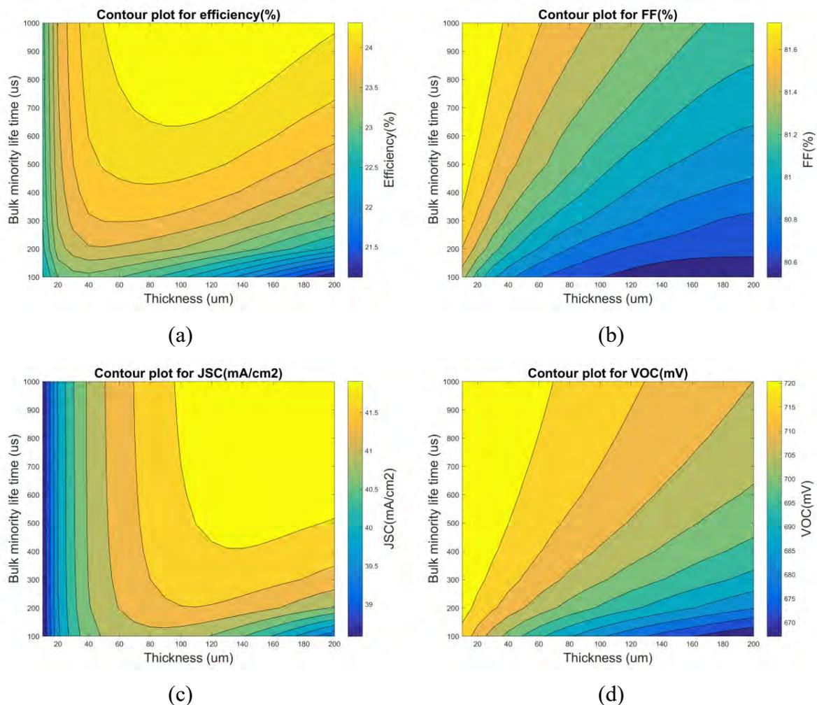
**Figure 3 Quokka simulation results for cell efficiency, fill-factor, open circuit voltage and short circuit current for different cell thickness and bulk minority lifetime.**
