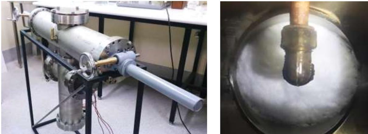
**Figure 5. The hydrate vessel and hydrate seen through the top view port.**
