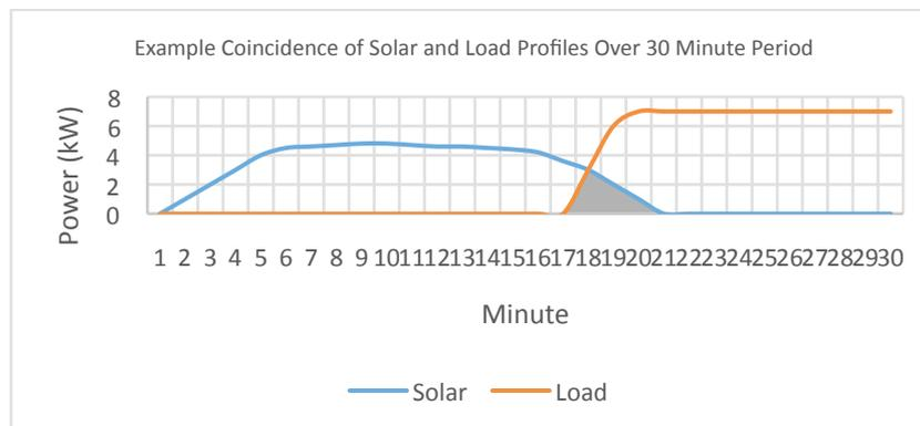
**Figure 1. Example Coincidence of Solar and Load Profiles Over 1 to 30 Minutes.**
