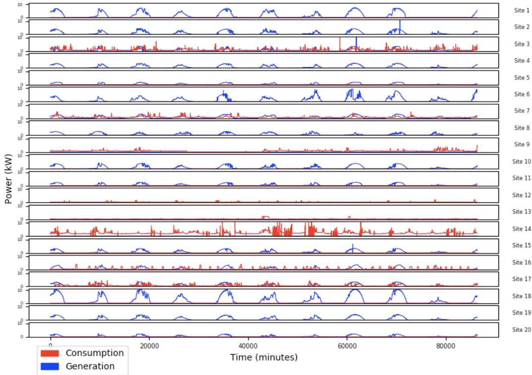
**Figure 2. Time Series Generation and Consumption at Measured Sites for a Sample 10 Day Period.**
