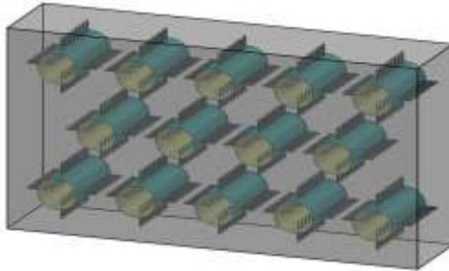
**Figure 2. High temperature finned heat pipe system**
