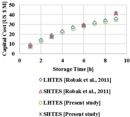
**Figure 3. Comparison of capital costs for the LHTES and SHTES for different storage times. The power generation is 50 MWe.**
