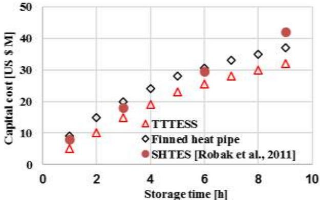
**Figure 4. Capital costs for TTES and Finned heat pipe system compared with a SHTES for different storage times. The power generation is 50 MWe.**
