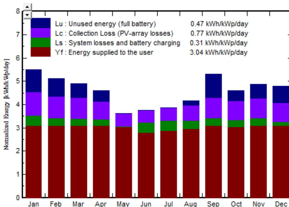
**Fig 4.2: Normalized PV production (per installed kWp): Nominal power 20.1 kWp**
