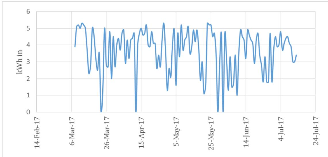
**Fig 4.3: Input energy from solar panels to batteries over a period of 3 months**
