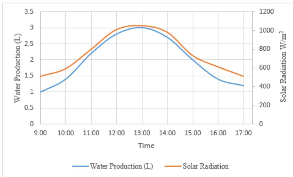
**Fig 4.1: Water production compared with the hourly solar radiation**
