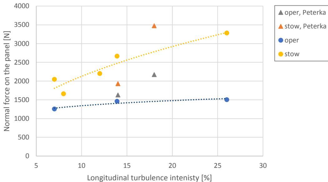
**Figure 6 The peak normal force on the mirror panel at maximum operating and stow speeds for a 7.22 m<sup>2</sup> heliostat as a function of turbulence intensity**
