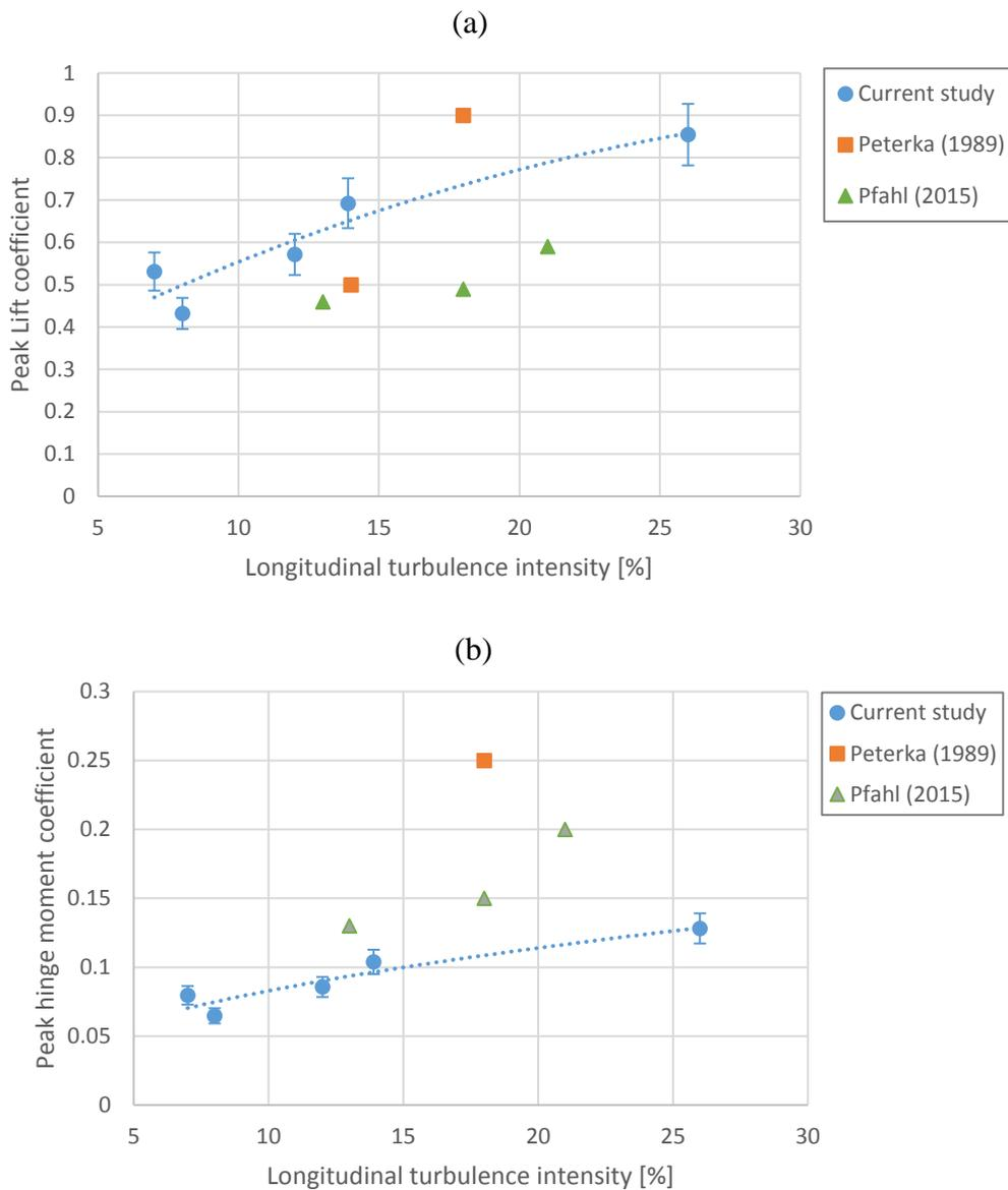
**Figure 4 The effect of longitudinal turbulence intensity on (a) peak lift coefficient (b) peak hinge moment coefficient on a stowed heliostat**
