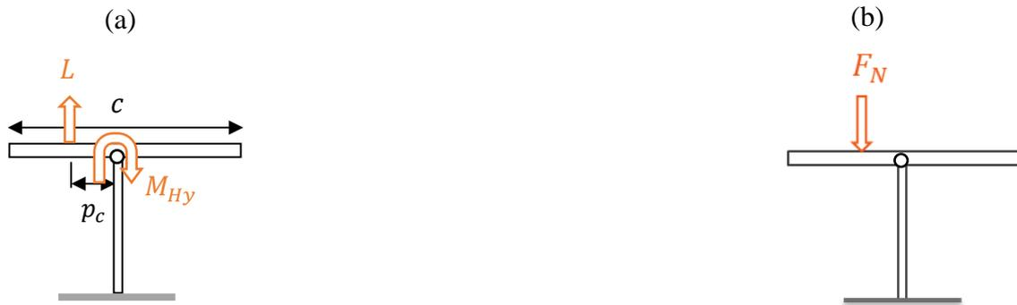
**Figure 3 (a) Main wind loads on a heliostat at stow position (b) Normal force on the stowed mirror panel**
