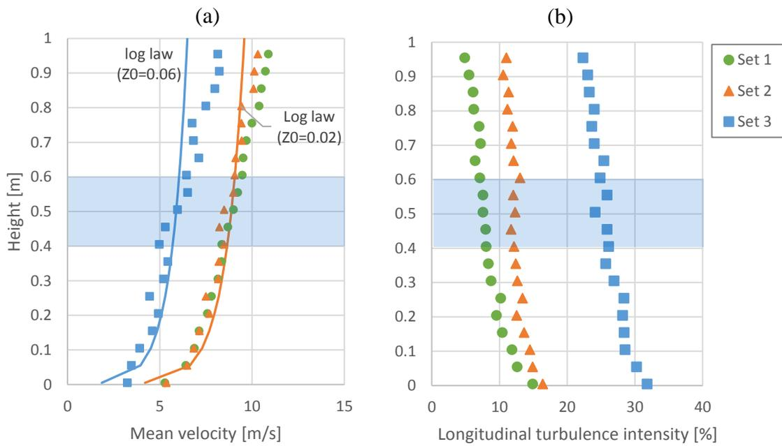
**Figure 2 (a) Mean velocity profile (b) Longitudinal turbulence intensity profile**
