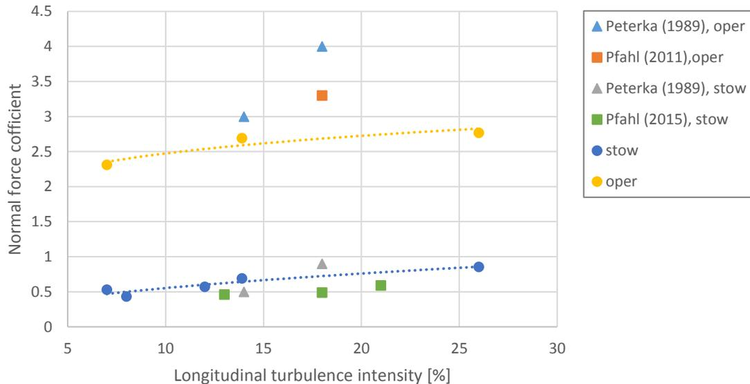
**Figure 5 Peak normal force coefficient at stow and operation as a function of turbulence intensity**
