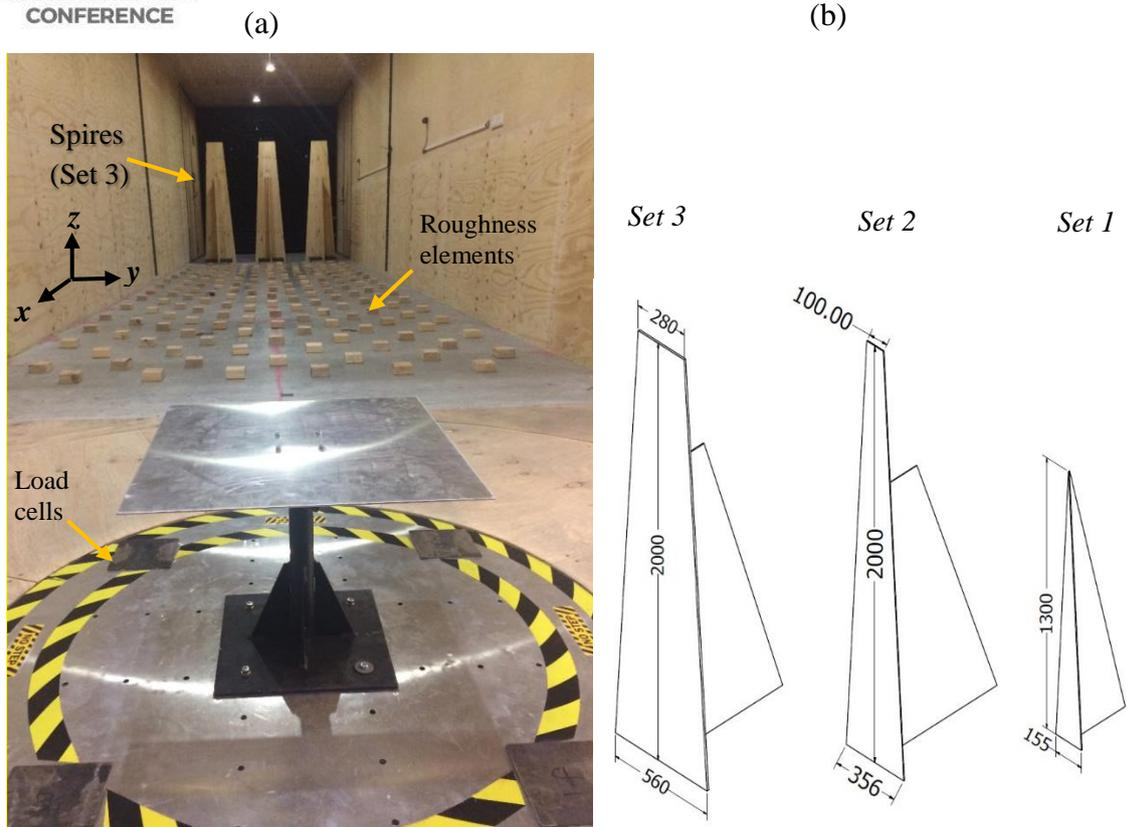
**Figure 1 (a) Experimental test setup (b) Dimensions of the three spire sets (in mm)**
