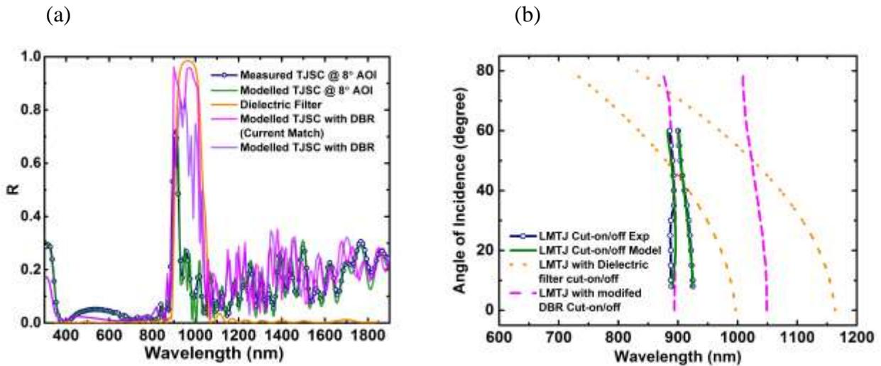
**Figure 4. (a) Measured and modelled specular reflectance of a lattice-matched TJSC with intermediate DBR, and reflectance of the TJSC with an intermediate DBR design for spectrum splitting. (b) AOI response of intermediate DBR in a TJSC versus a band-reflect dielectric filter.**
