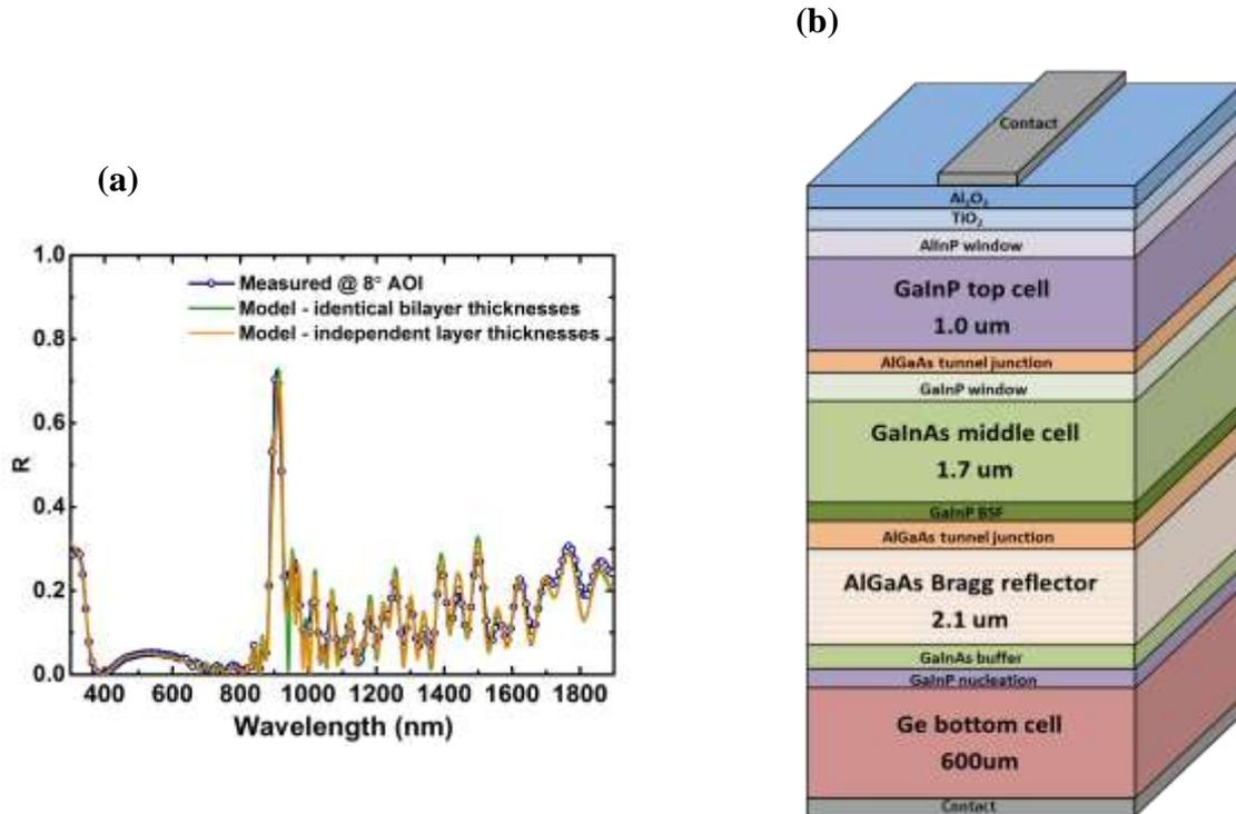
**Figure 3. (a) Modelled and measured specular reflectance of an Azur Space 1-sun terrestrial lattice-matched TJSC with intermediate DBR. (b) Schematic cross-section of the LM TJSC structure (not to scale).**
