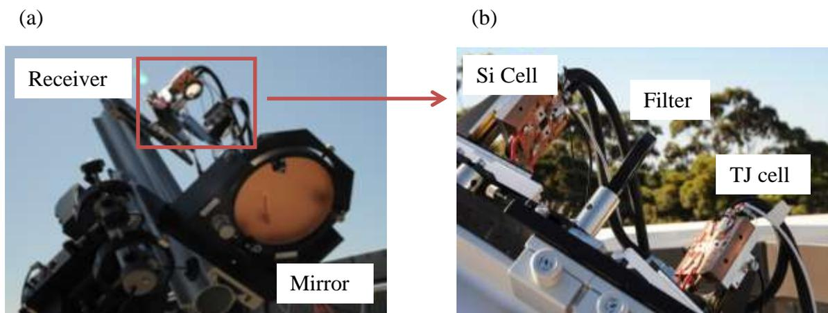
**Figure 2. (a) Photograph of the prototype, (b) close-up of the 'receiver' in the prototype.**
