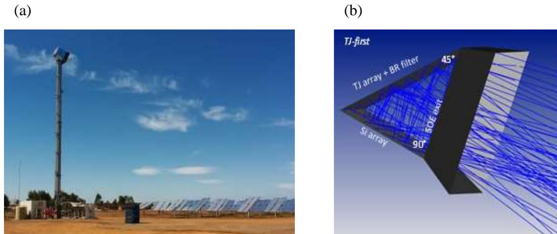
**Figure 1. (a) RayGen's central receiver CPV power tower system. (b) Schematic of a V-shaped spectrum-splitting receiver, relevant to this project.**
