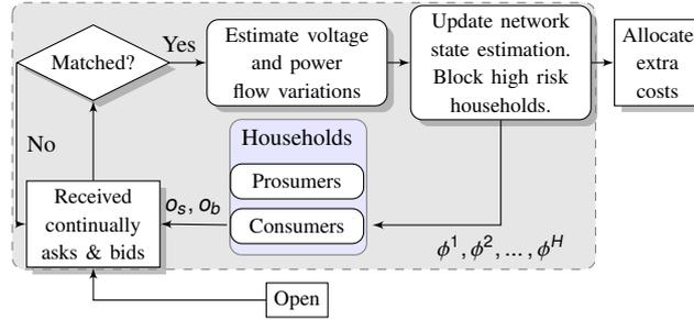
**Figure 4:** Schematic of the P2P trading under network constraints.
