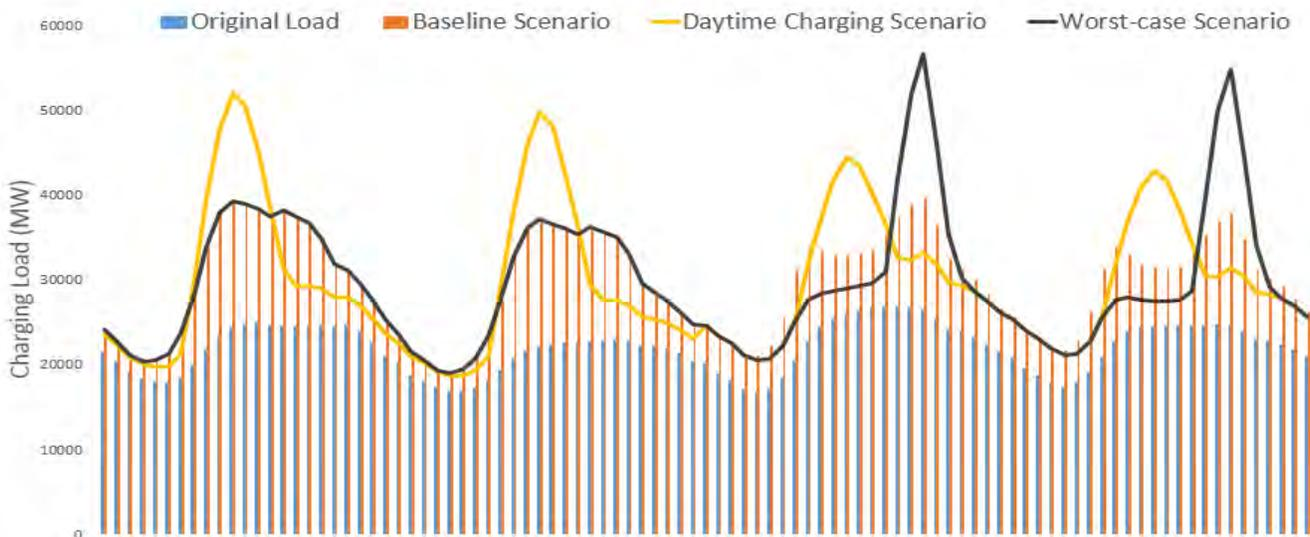
**Figure 1. Plot of different charging regimes and original load over the first 4 days of the modelled period (01/01/2006 1am – 04/01/2006 11pm)**
