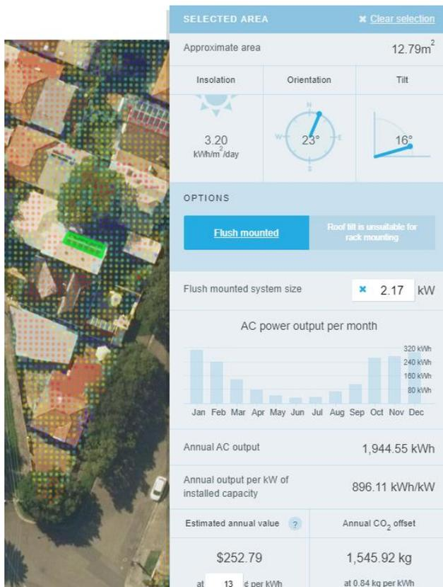
**Figure 3: SunSPoT output for selected roof section**
