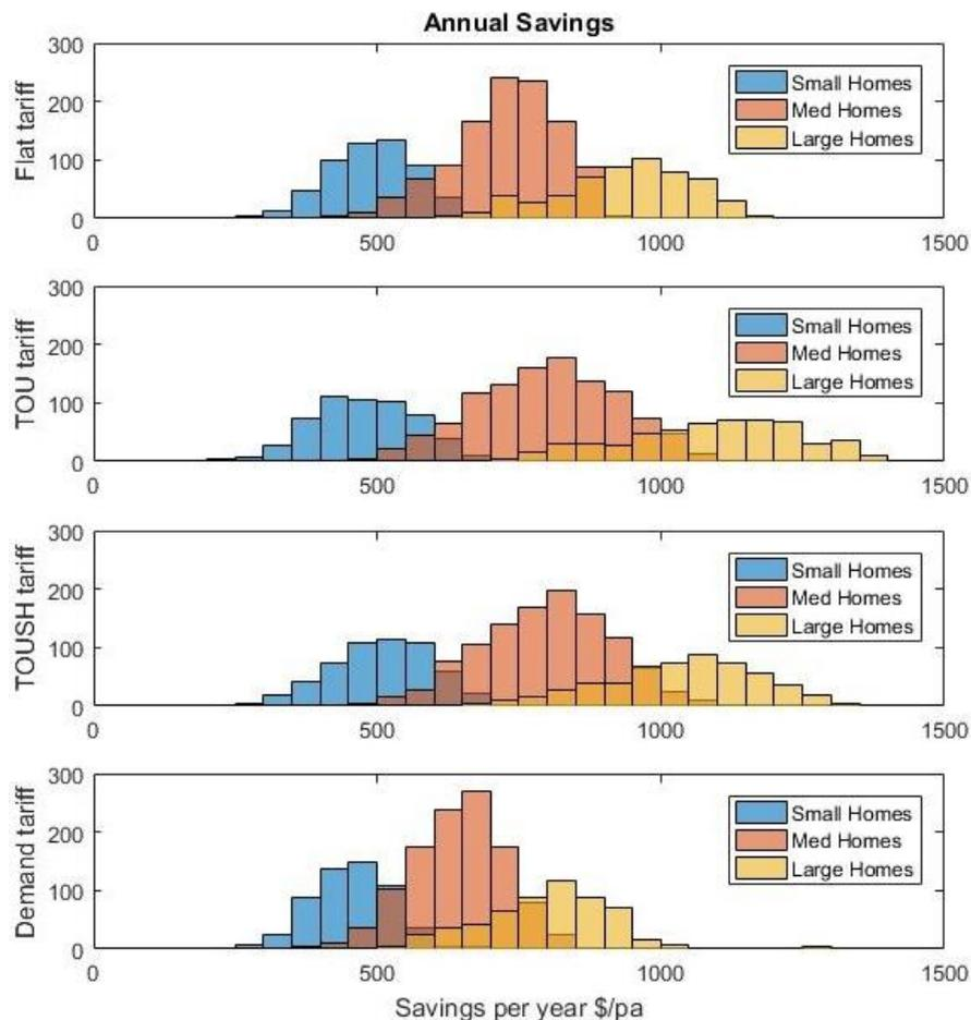
**Figure 2: Savings per annum for medium PV and medium storage scenario, with overlap in distributions visible**
