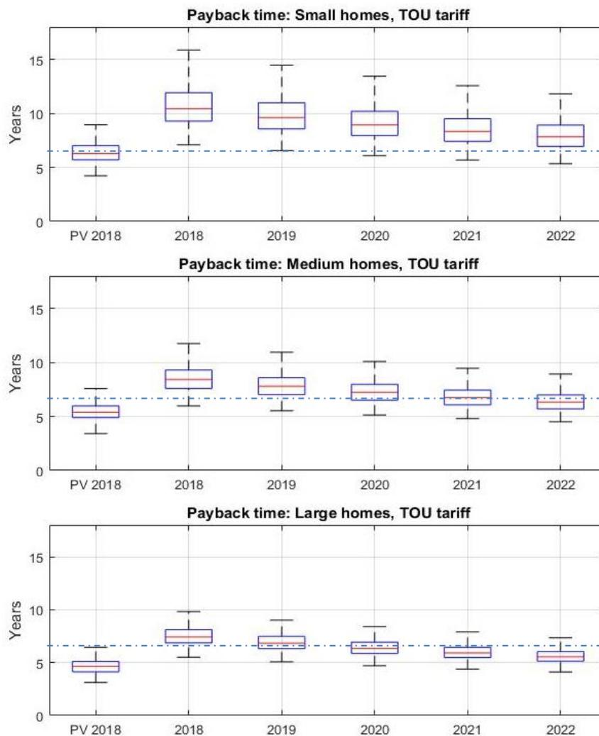
**Figure 4: Payback times for homes on a TOU tariff with a large PV system and a small battery**
