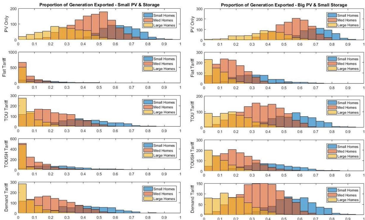
**Figure 3: Distribution of percentage of PV generation exported by small, medium and large households under different BES operation methods in a small PV and BES scenario (left) and a large PV and small BES scenario (right)**
