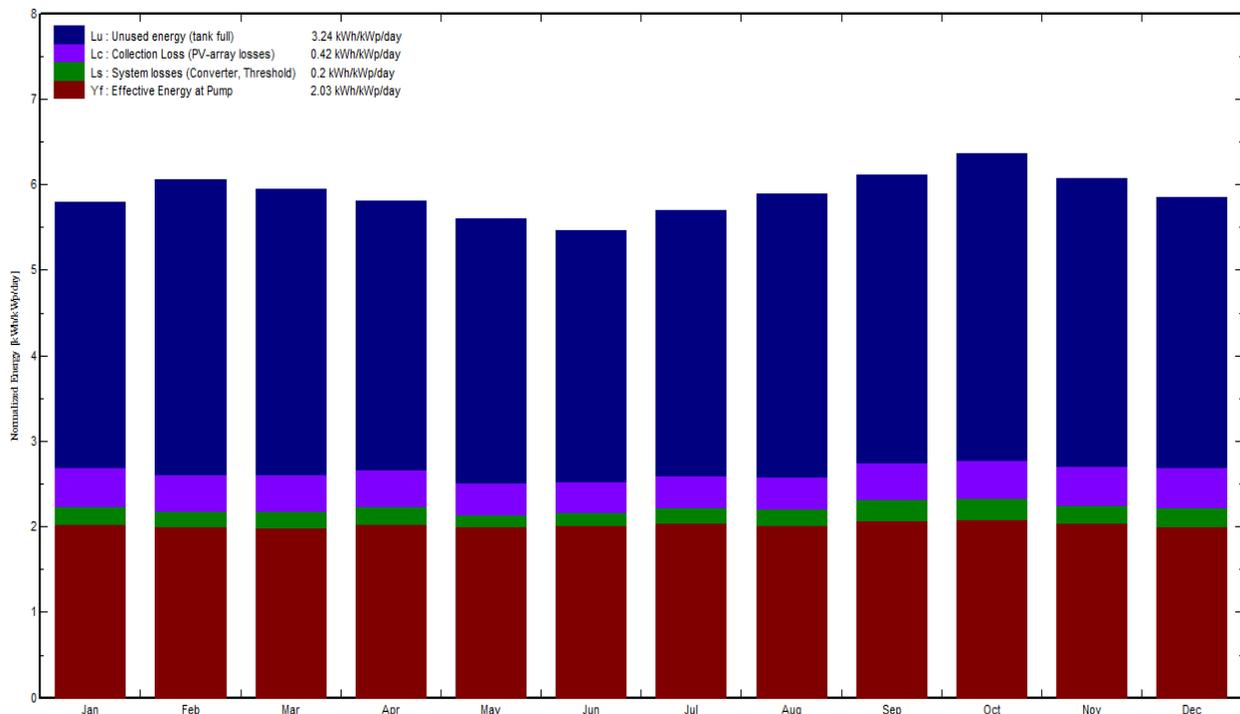
Figure 4. Normalized productions per installed kWp.
