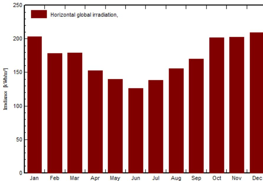
**Figure 2. Average solar irradiation in Namau area ( $17.61^{\circ}$  South and  $177.79^{\circ}$  East)**
