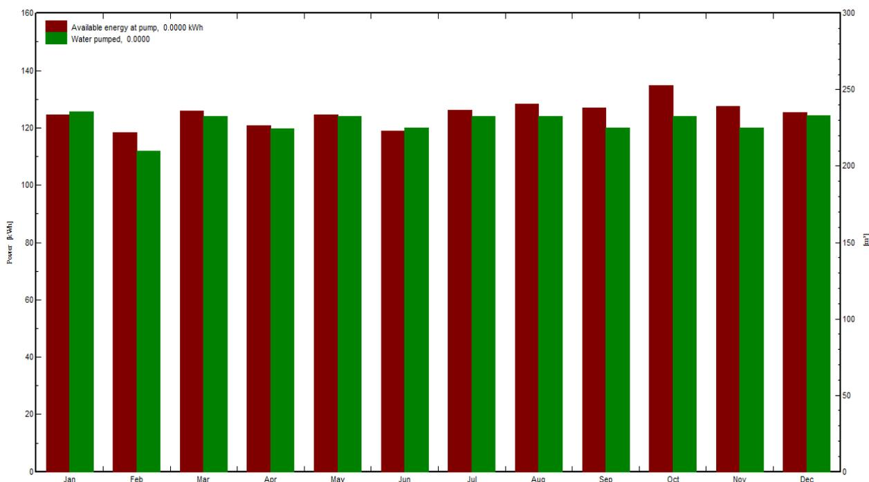
Figure 5 : Available energy at the pump versus water pumped over the year
