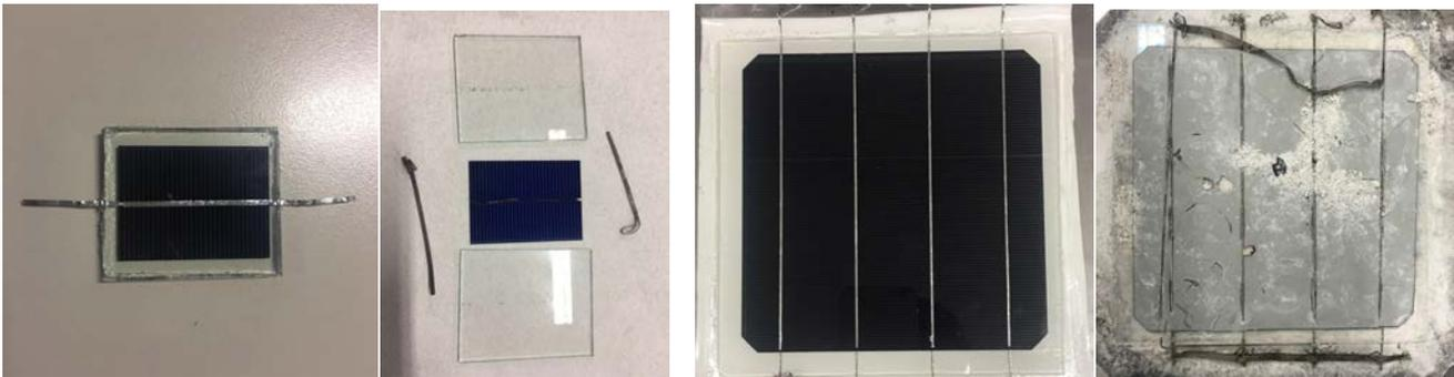
Results shown that the thermal process requires a precisely designed heating profile that can eliminate the volume of released gas due to decomposition of EVA. Hence, several heating programs were developed and tested, including step-heating and repeated-heating profiles to minimize sudden and large production of gases. However, further research is required to minimize the breakage issue with thermal processes.
