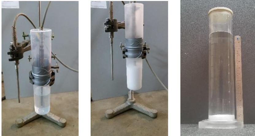
**Figure 1. 80mL sample of PCM subjected to cycling tests (left and centre) and 2500mL of -6PCM failure due to separation (right).**
