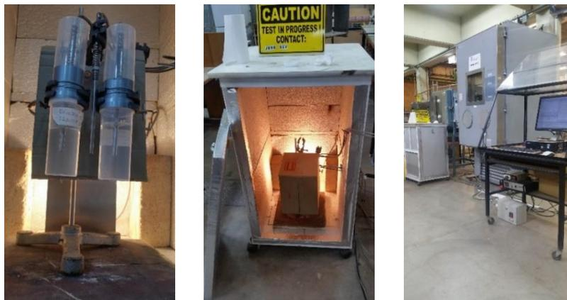
**Figure 2. Pseudo T-history setup with the sample, reference and ambient temperature measurements shown on the left, the constant room temperature enclosure centred and the constant temperature freezer with controllers shown on the right.**
