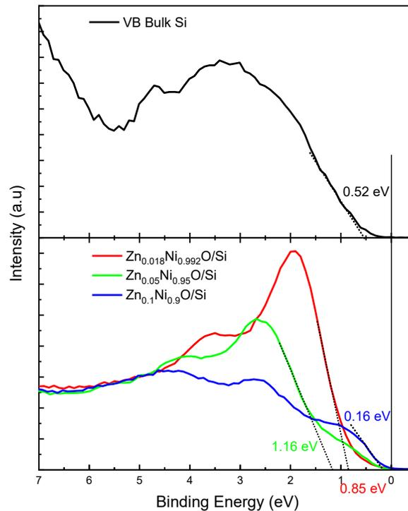
**Figure 1. The valence band spectra of a bare Si and the Zn<sub>x</sub>Ni<sub>1-x</sub>O (x = 0.018, 0.05, 0.1) films deposited onto silicon substrate.**
