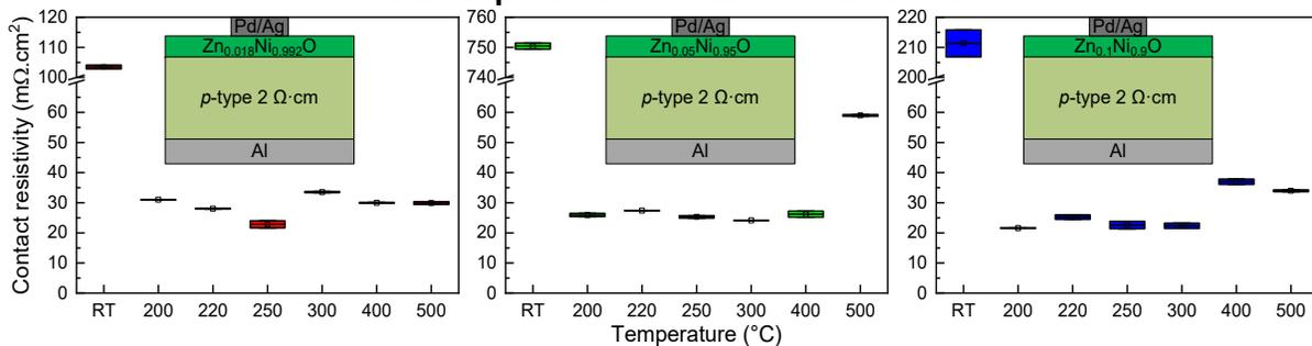
**Figure 2. Contact resistivity of the Zn<sub>x</sub>Ni<sub>1-x</sub>O (x = 0.018, 0.05, 0.1) films onto p-Si before and after annealing.**
