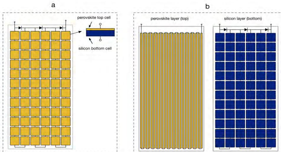
Figure 1. Cell shapes and connection configurations for (a) 2T and (b) 4T PSC/Si tandem-cell modules.
