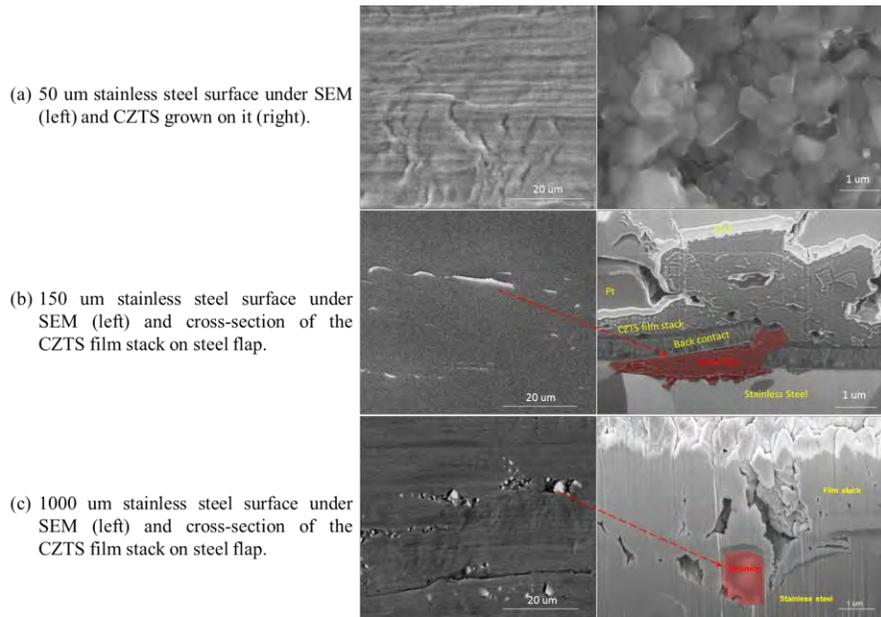
**Figure 1. Surface morphologies of different stainless steels and cross-section of CZTS film stack on different surface defects.**
