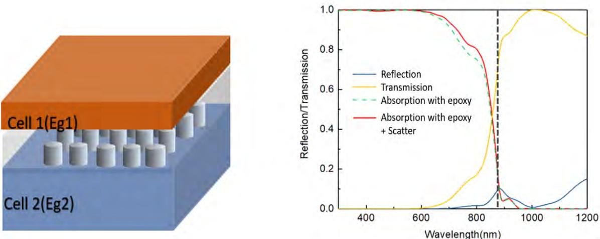
**Figure 1. (a) Illustration of intermediate layer consist of scatter array and transparent epoxy. (b) Transmission, reflection and absorption spectra for III-V MJSCs with/without scatter.**
