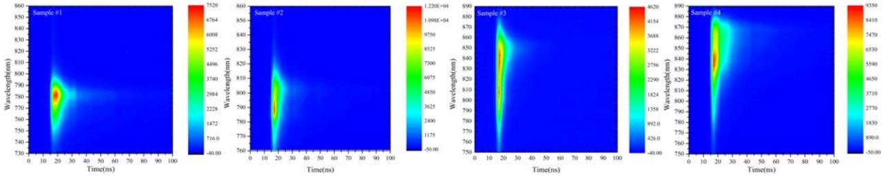
**Figure 1: TCSPC 2D plots for samples 1 to 4 with varying quantum well width. Excitation wavelength is 640nm and time resolution is 66ps. A clear evolution of the spectral shape with time is evident, especially for the wider wells.**
