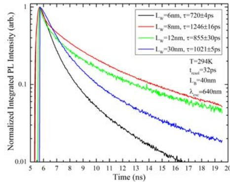
**Figure 3: Integrated PL intensity with time delay for samples with varying well width.**
