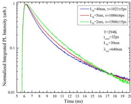
**Figure 2: Integrated PL intensity with time delay - samples with varying barrier width.**
