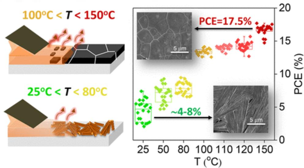
**Figure 1** Schematic diagram of blade coating at different temperatures. A plot of blade coating temperature vs. power conversion efficiency of the devices with SEM images as inset. Higher coating temperature results in higher PCE and better reproducibility<sup>2</sup>.
