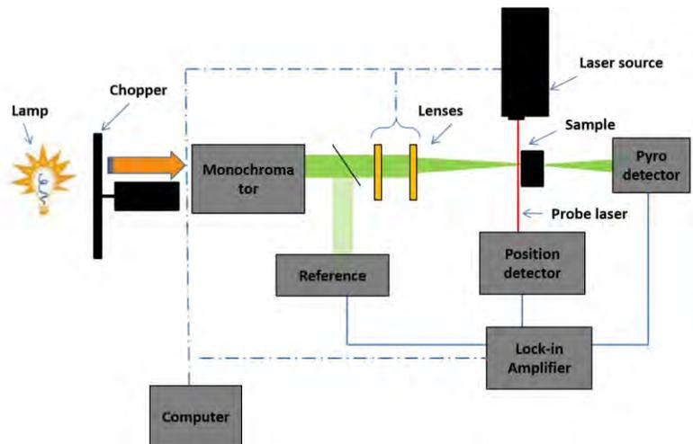
Figure 1: The PDS setup block diagram
