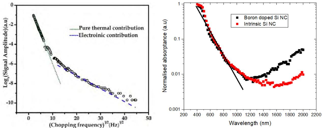
Figure 1: (left) Thermal vs Electronic contribution to PDS signal on a silicon sample, (right) Normalised PDS signal from silicon nanocrystal sample.
