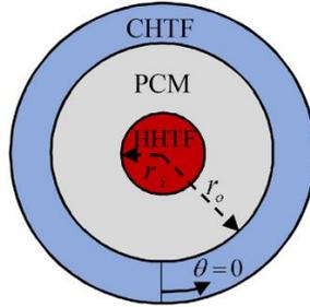
**FIGURE 8.** The schematic of the triplex tube heat exchanger.
