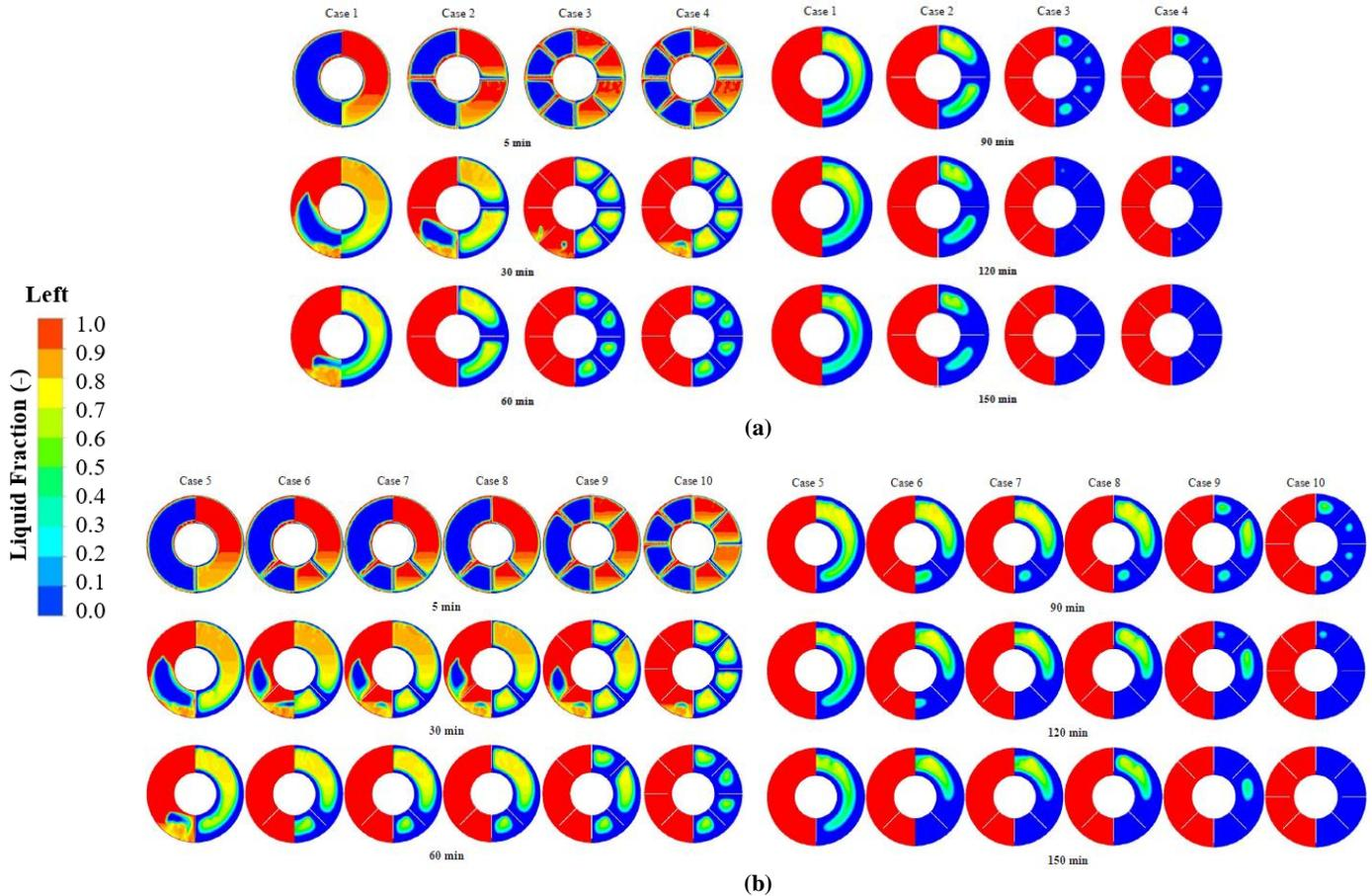
**FIGURE 10.** Liquid fraction contours for (a) conventional and (b) developed fin configurations under melting (left) or solidification (right) from both sides.
