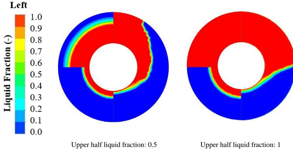
**FIGURE 5.** Logic verification where each contour shows the CCNC model (right) and the corresponding novel method results (left)
