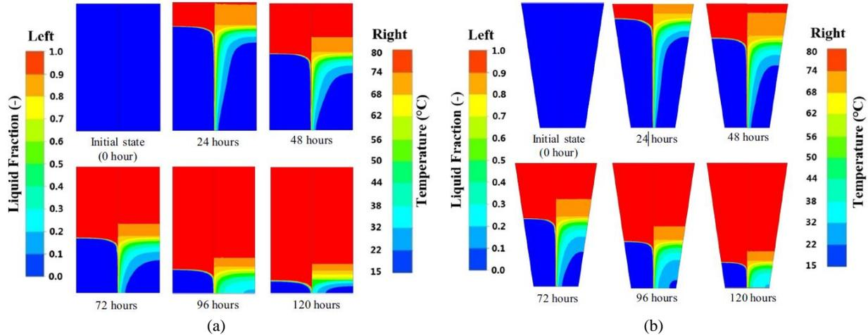
**FIGURE 3.** The contours of the PCM liquid fraction (left) and temperature (right) in the (a) cylindrical and (b) conical systems during charging
