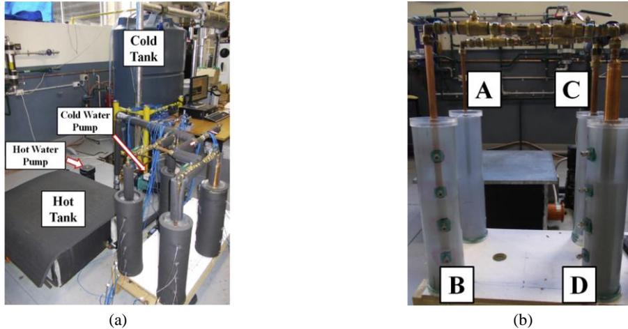
**FIGURE 6.** Pictorial views of (a) the whole experimental rig (b) the four PCM storage cylinders
