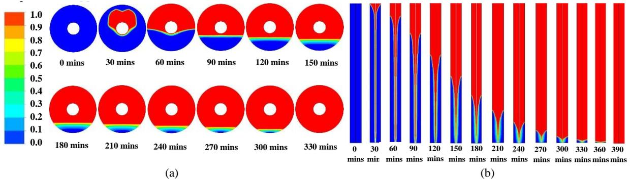
**FIGURE 4.** Contours of PCM liquid fraction during charging process in (a) horizontal and (b) vertical units
