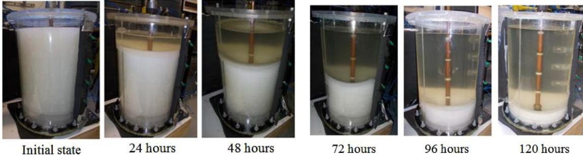
FIGURE 2. Evolution of the liquid/solid PCM interface at different charging times
