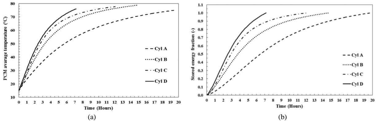
**FIGURE 7.** Comparison of the (a) PCM average temperature, and (b) stored energy fraction during the charging process
