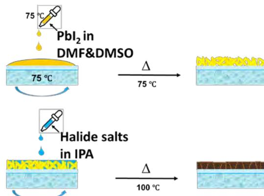
**Figure 1.** Schematics of two-step sequential deposition processes of fabricating mesoporous  $\text{PbI}_2$  films and perovskite film.
