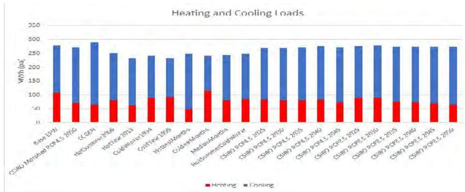
Figure 1. Changes in Annual Heating and Cooling Loads for different Weather Data Sets
