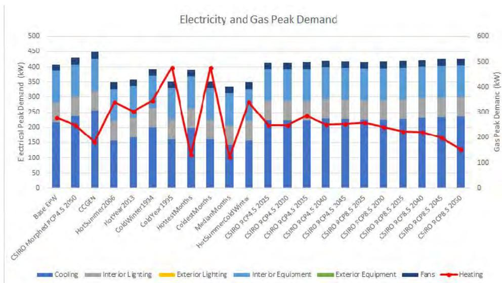
**Figure 3. Electricity and Gas Peak Demands for different Weather Data Sets**
