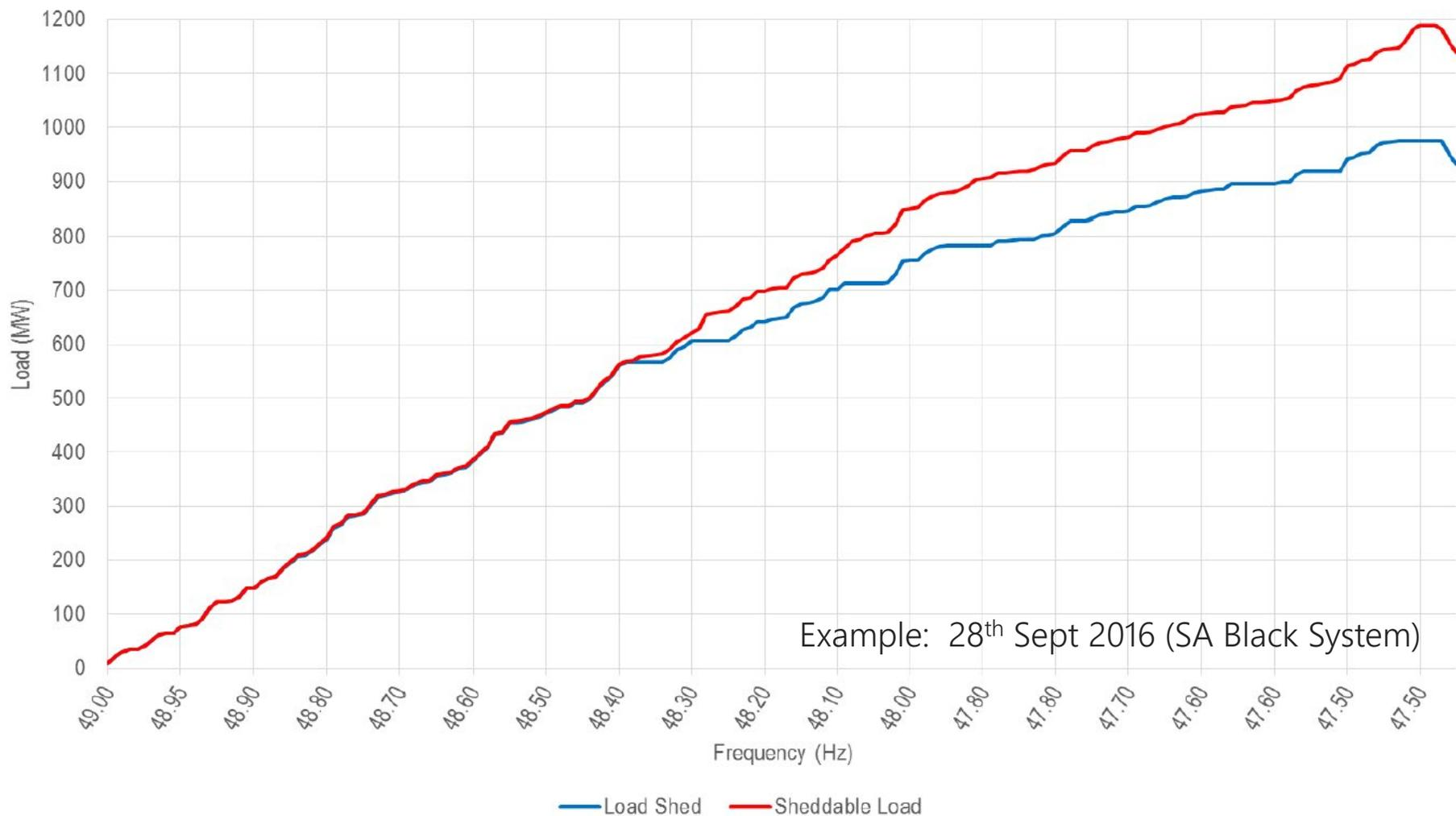
As frequency falls, load is progressively shed in an attempt to stabilise the system.
