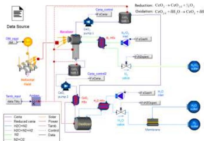
Figure 1: Modelica component diagram of the thermochemical production plant.
