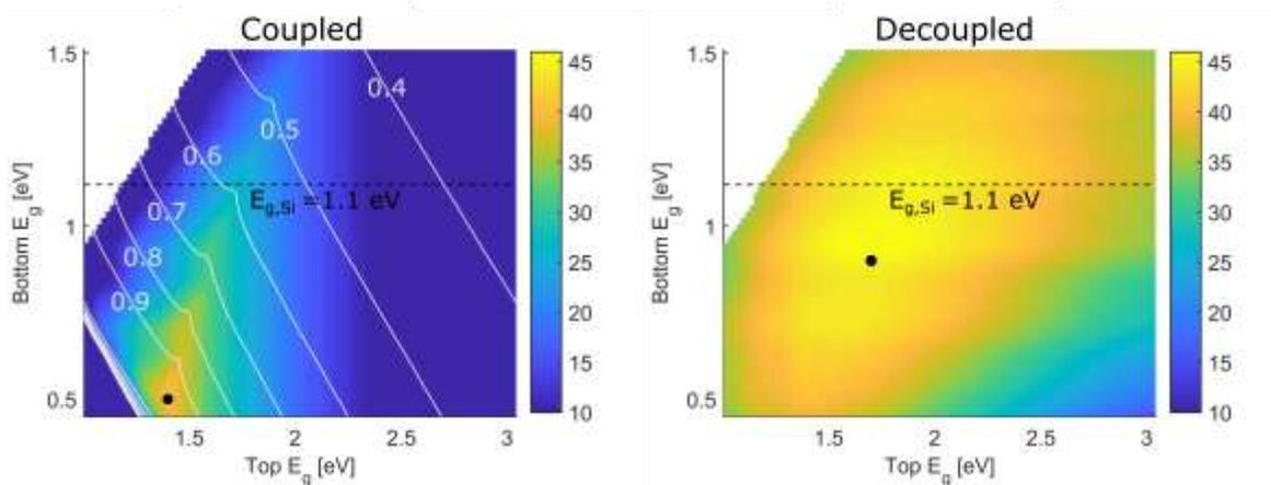
**Figure.2 Ideal solar-to-hydrogen (STH) efficiency limits [%] for coupled and decoupled tandem PV water splitting systems, for different semiconductor bandgaps. The white contour lines indicate the ratio of the STH and PV efficiencies.**
