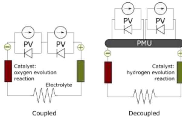
**Figure 1: Equivalent circuit diagrams for coupled and decoupled tandem PV water splitting systems.**
