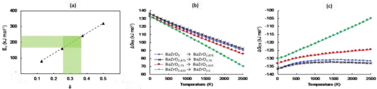
**Figure 2.** (a) PBE-PAW  $E_v$  values (per defect) of  $\text{BaZrO}_{3-\delta}$  as a function of oxygen non-stoichiometry  $\delta$ . The green region indicates the optimum  $E_v$  range of 170 – 230 kJ mol<sup>-1</sup> (1.8-2.4 eV).<sup>4</sup> The change in Gibbs free energy of (b) reduction reaction,  $\Delta G_{RR}(T, p)$  (equation (6)) and (c) oxidation reaction,  $\Delta G_{OR}(T, p)$  (equation (7)).
