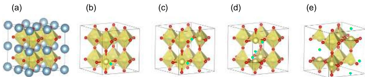
**Figure 1.** 2x2x2 supercells of (a) pristine BaZrO<sub>3</sub> (b) BaZrO<sub>2.875</sub> (c) BaZrO<sub>2.75</sub> (d) BaZrO<sub>2.625</sub> (e) BaZrO<sub>2.5</sub>. Grey, gold and red spheres represent Ba, Zr and O atoms, respectively. (b)-(e) omit Ba for clarity. Green spheres represent position of oxygen vacancy defect in (b)-(e). Gold surfaces indicate ZrO<sub>3</sub> octahedra.
