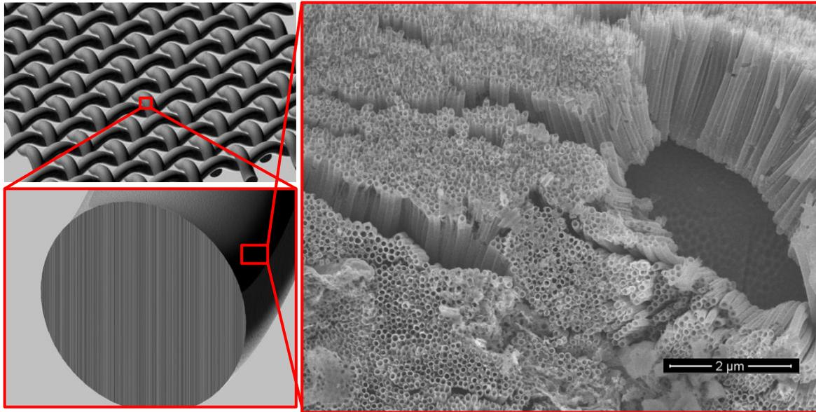
**Figure 1. Electrode structure of anodically grown, amorphous TiO<sub>2</sub> nanotube arrays hierarchically grown on a titanium mesh substrate, for use as a Lithium Ion Capacitor anode**
