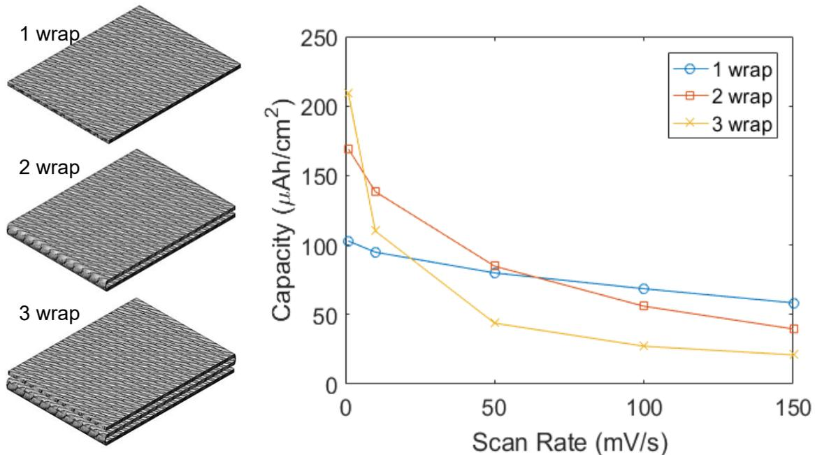
**Figure 2. Capacity retention (as indicated by cyclic voltammetry) at higher scan rates for an unoptimized scaling method, showing poorer retention for the stacked, 3d electrode (“3 wrap”) than for the analogous single layer, research style (“1 wrap”) electrode**
