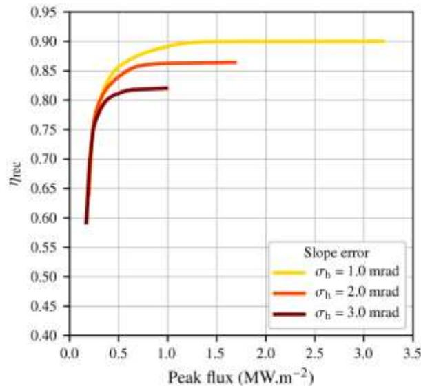
**Figure 2: Pareto fronts highlighting the design trade-off between peak flux and receiver efficiency for cylindrical molten salts receivers on the ASTRI field system.**
