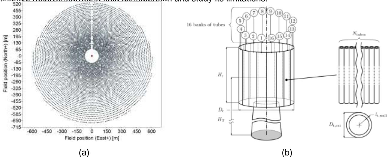
**Figure 1. ASTRI's reference heliostat field using a "gear staggered" layout and (b) Receiver geometrical model in this study.**
