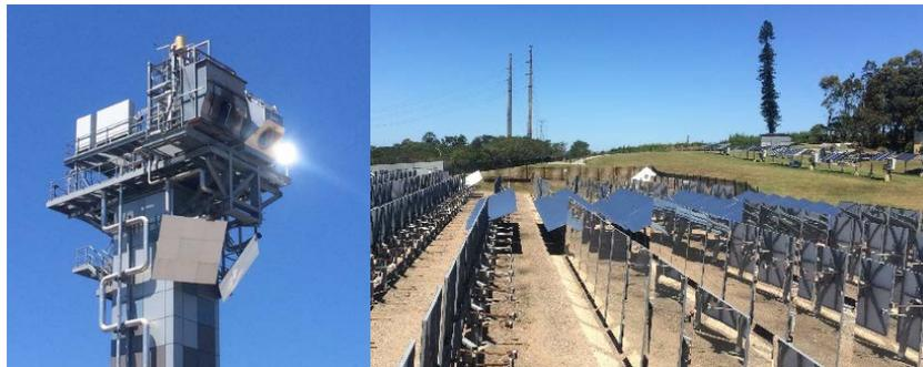
**Figure 2. Camera Array Calibration System measuring reflected images of 30 heliostats simultaneously**
