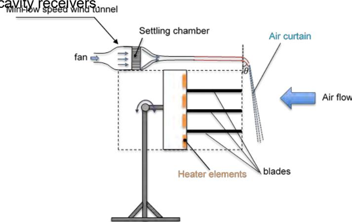
**Figure 1. Schematic of experimental rig located in the wind tunnel at the University of Adelaide**
