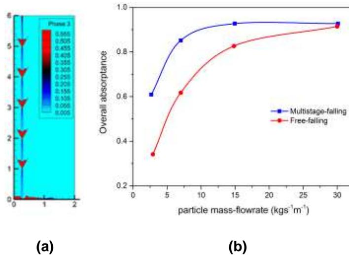
**Figure 1. Eulerian-Eulerian CFD modelling of multistage free-falling particle receiver: (a) particle volume fraction for V shape troughs and (b) overall absorptance**
