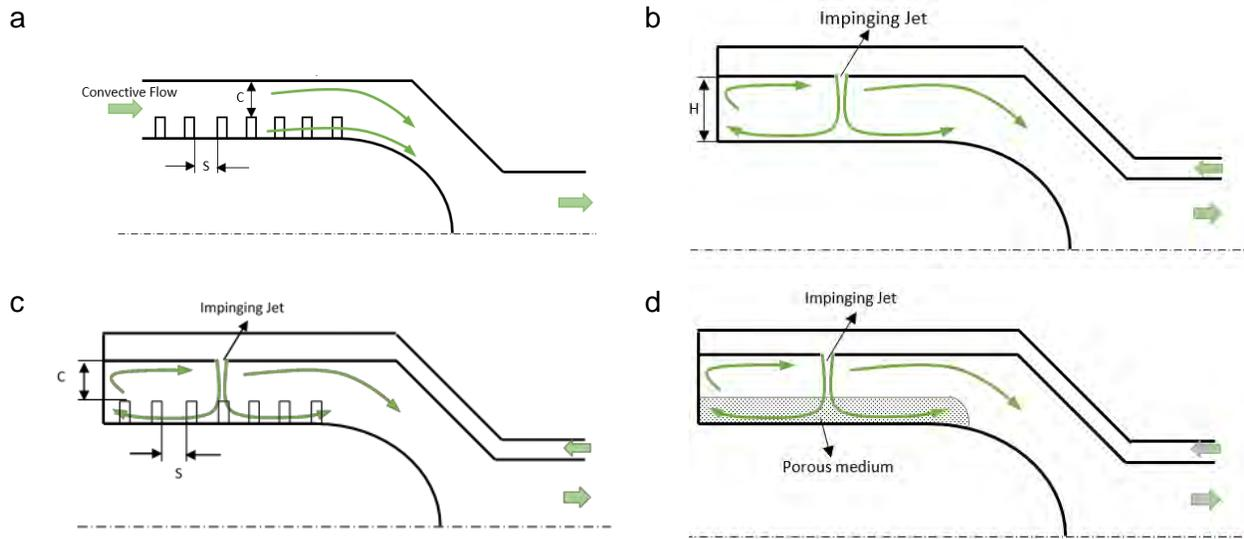
Figure 1 Schematic of the models analysed in this paper: (a) plate-fin under convective flow; (b) clean cavity (or roughened cavity) exposed to impinging jets; (c) cavity with plate-fin exposed to impinging jets; (d) cavity with porous medium exposed to impinging jet.
