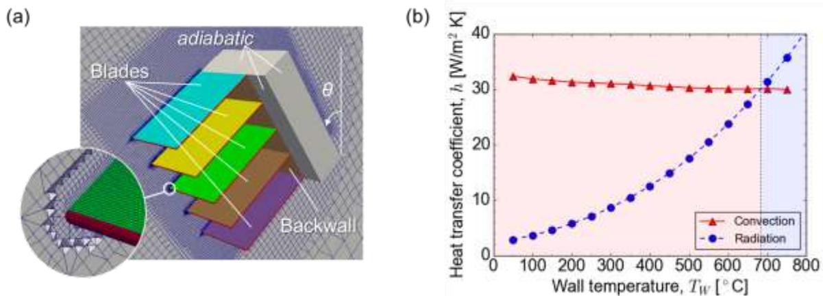
**Figure 1. CFD model (a) and heat transfer coefficient as a function of wall temperature for a bladed structure with five blades, aspect ratio  $R_{BS} = 5$ , and wind speed  $U = 5$  m/s (b)**
