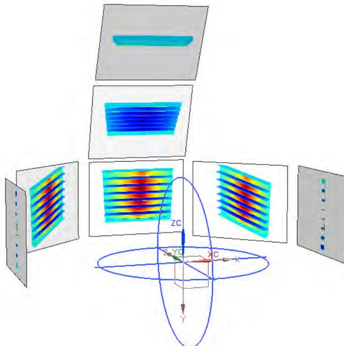
**Figure 1. Radiosity distribution from a multi-cavity receiver, bladed receiver, which is viewed in different directions that cover the hemisphere**
